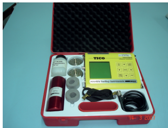
Figure 4. PUNDIT-Portable Ultrasonic Non-destructive Digital Indicating Tester
