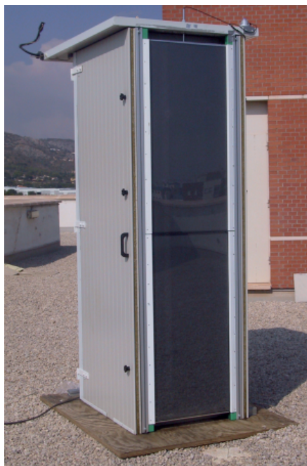
Figure 5. Front view of the ventilated envelope prototype.
