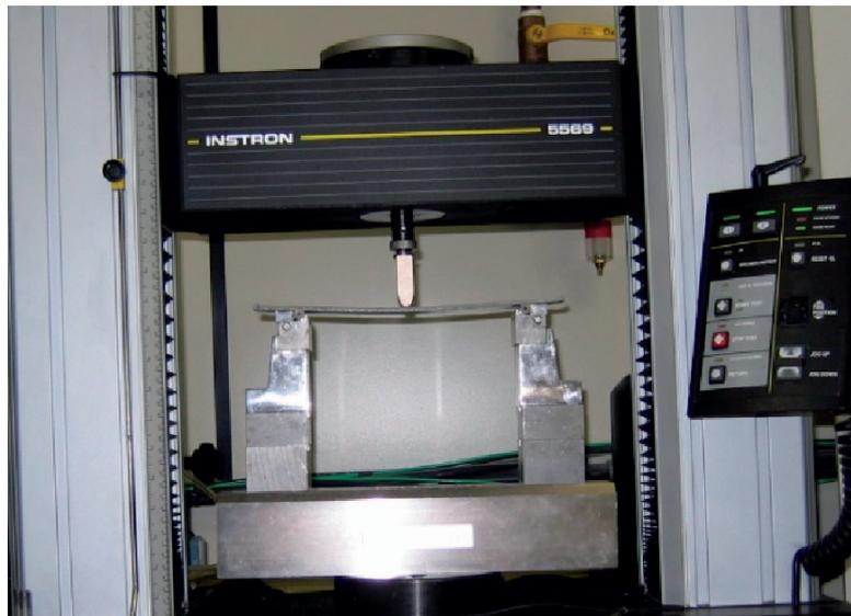
Figure 3. Configuration of the test using the experimental programme for measuring flexibility.
