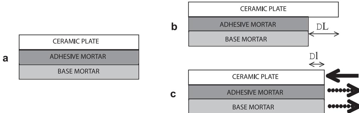
Figure 2. Diagram of acting stresses on the system due to the action of water on the ceramic Tilings (a – dry condition; b – plate water saturation (free layers – hypothetical); c – real behaviour owing to solidarity between layers).
