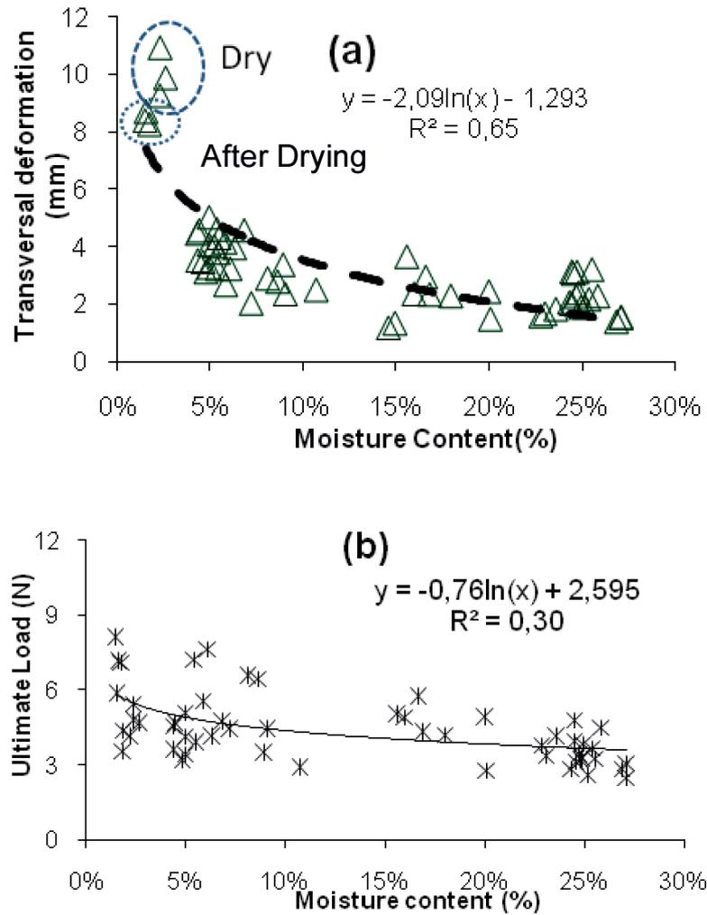
Figure 6. Results for the transversal deformation test. (a) Flexibility and (b) Ultimate load.
