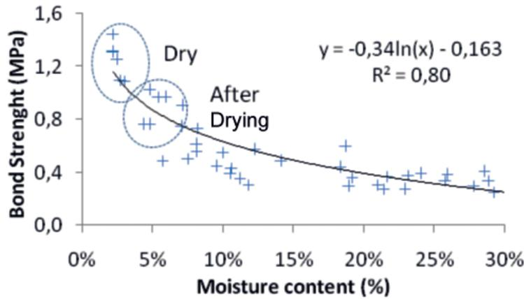
Figure 7. Bond Strength x Moisture Content.
