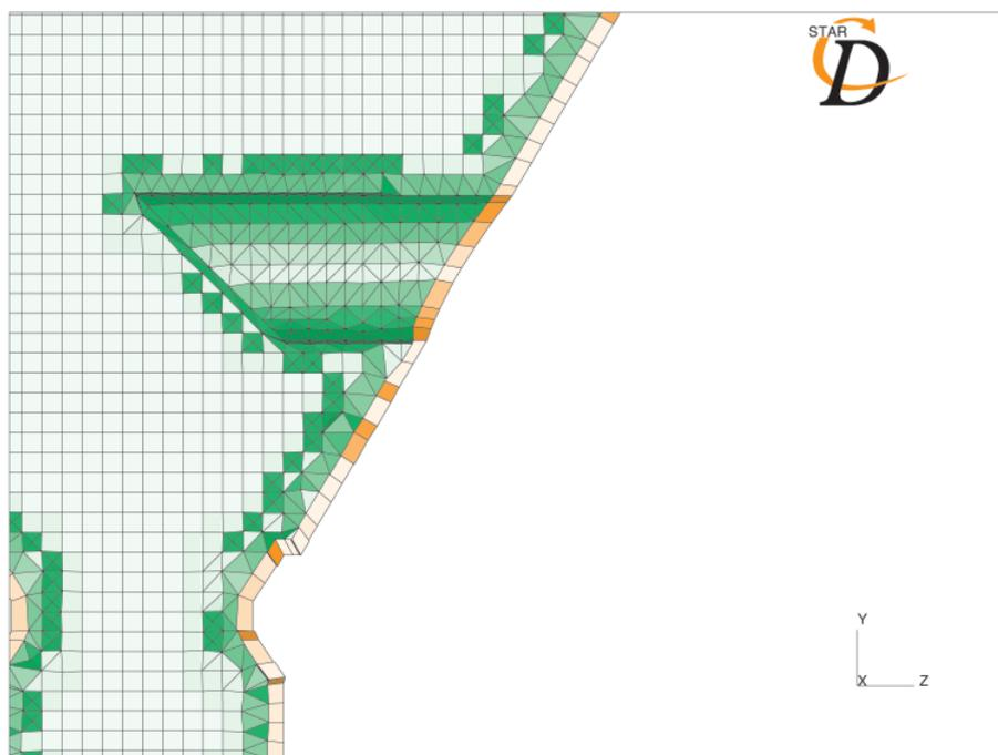
Figure 2. Detail of the volumetric mesh inside the chamber..
