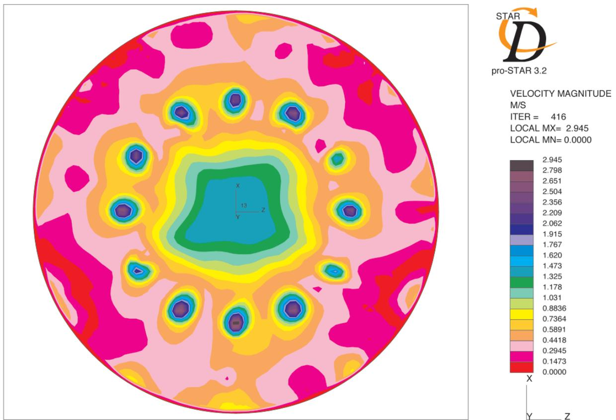
Figure 5. Velocity magnitude. Top view of the injection region..
