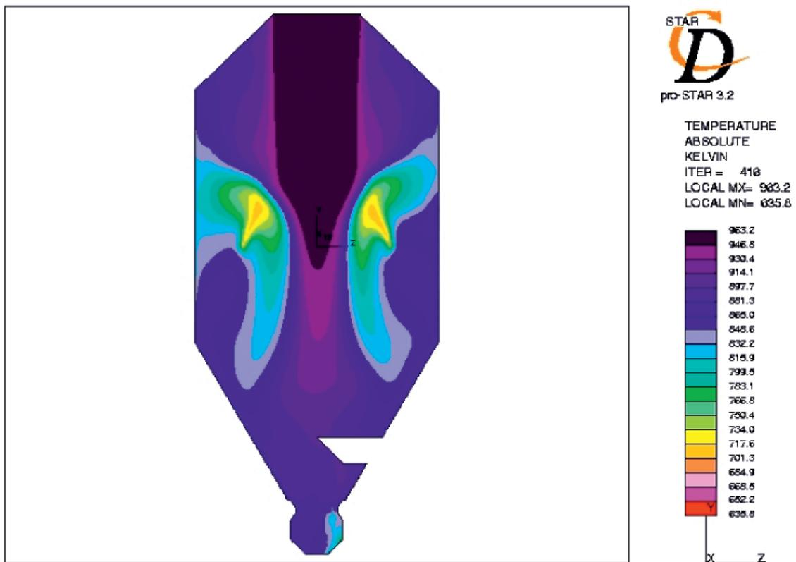
Figure 7. Temperature profile at the axis of the chamber, after injection of droplets.
