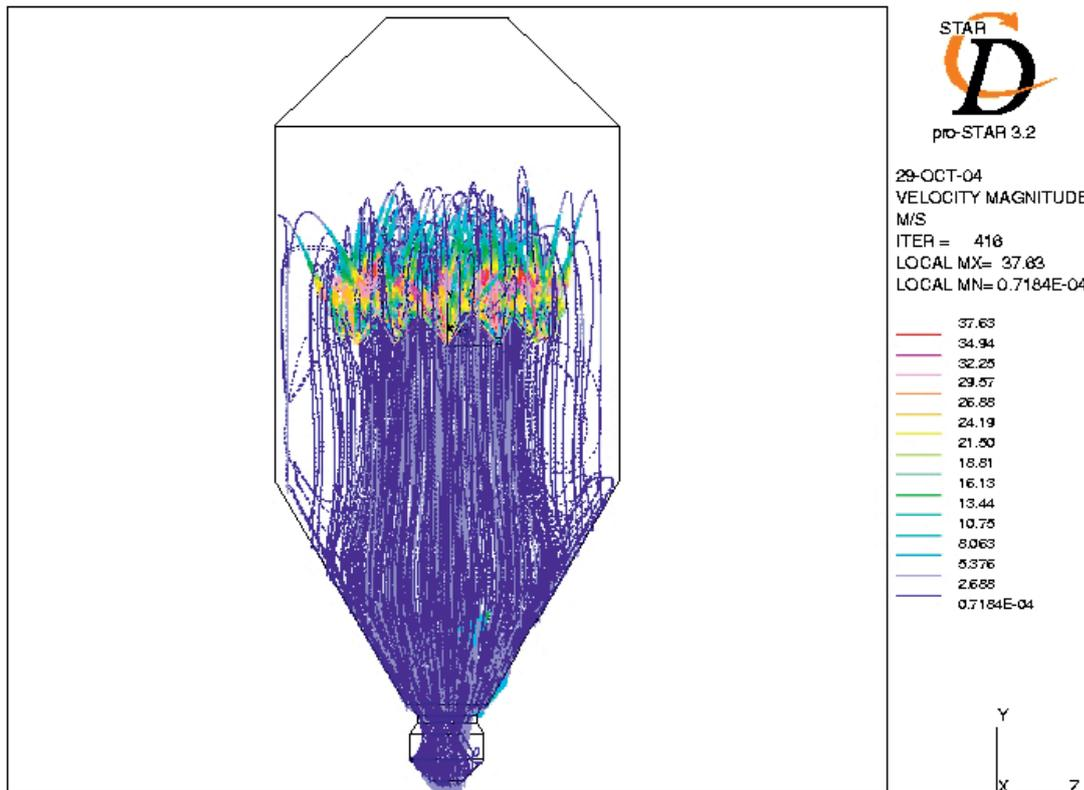
Figure 10. Droplets trajectories. Front view.
