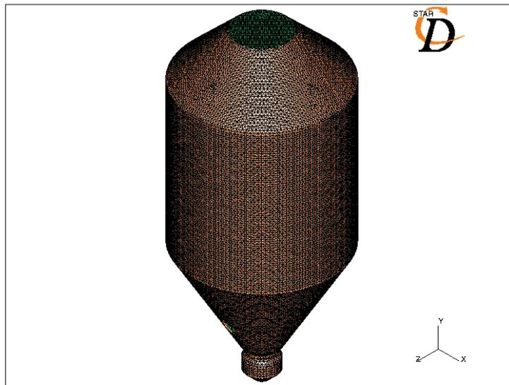
Figure 1. Meshed domain of the drying chamber.
