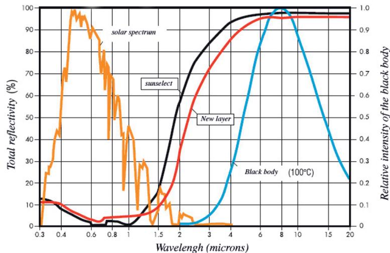
Figure 4. Spectral reflectivity of the new copper electro-deposited layer.
