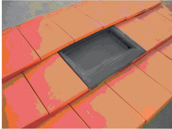
Figure 5. Designed encapsulating roof tile.
