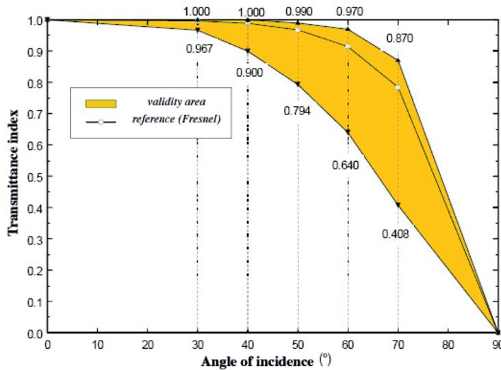
Figure 3. Transmittance of the selected glass with incident solar angle.
