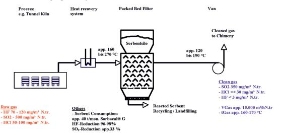
Figure 8. Conventional packed bed filter with granulated sorbent
