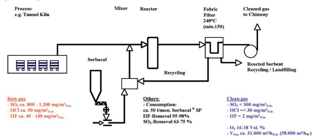
Figure 11. Dry sorption with fabric filter
