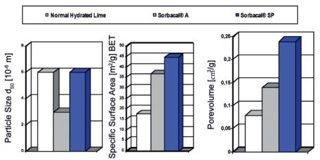
Figure 3. Comparison of different Hydrated Limes
