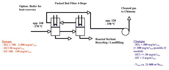
Figure 10. 4-stage packed bed filter system with temperature management
