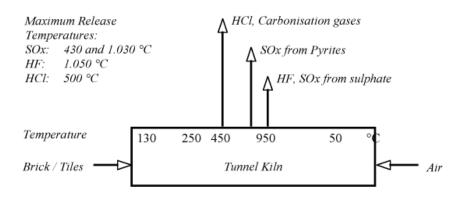
Figure 1. Release of pollutants in the ceramic process
