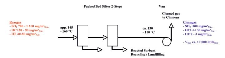
Figure 9. Multistage packed bed filter systems (2-stage)
