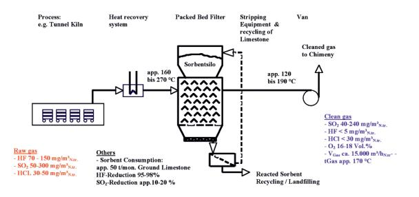
Figure 7. Conventional packed bed filter with ground limestone
