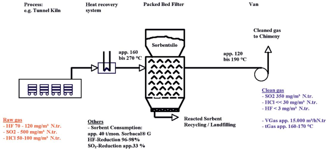
Figure 8. Conventional packed bed filter with granulated sorbent
