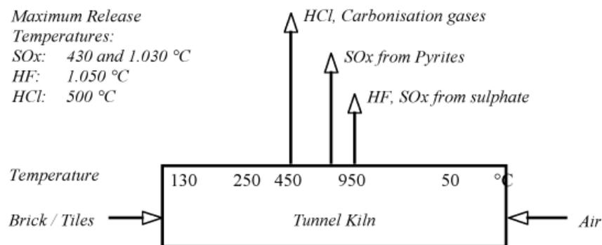
Figure 1. Release of pollutants in the ceramic process
