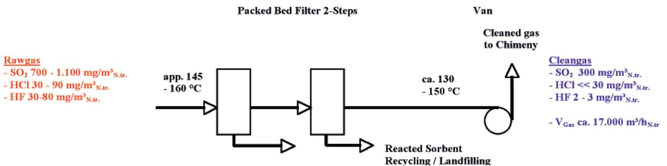
Figure 9. Multistage packed bed filter systems (2-stage)
