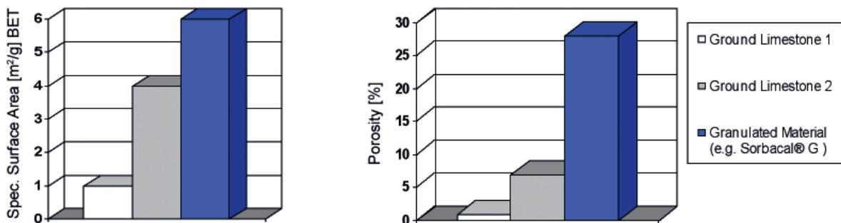
Figure 5. Specific surface area and porosity of ground limestone and granulated sorbent
