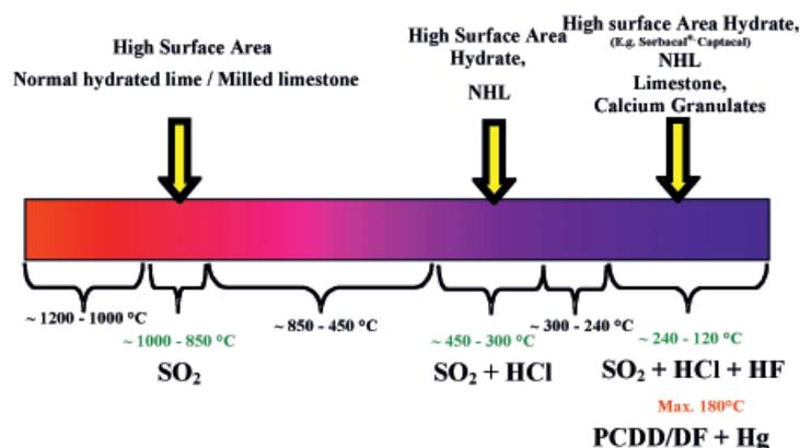
Figure 2. Temperature application range of FGT with lime based products
