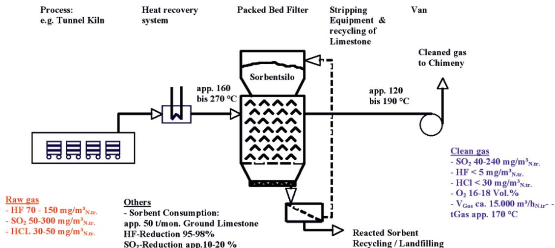
Figure 7. Conventional packed bed filter with ground limestone
