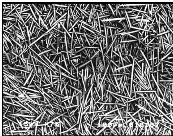
Figure 2. SEM micrograph related to amorphous silica fibres. Magnification: 75 X.
