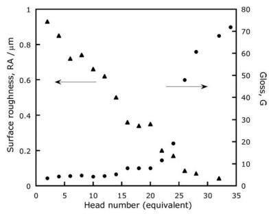
Figure 3. Data from Figure 2 re-plotted in terms of the equivalent number of polishing heads in an industrial line.
