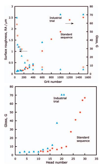
Figure 6. Evolution of surface roughness and gloss for tiles withdrawn from the industrial polishing line for the standard sequence of polishing steps (red points) and for the abbreviated sequence used in the trials (blue points):
