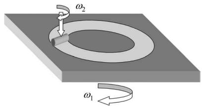
Figure 1. Schematic diagram of the laboratory-scale rig, showing the motion of the square tile sample (with rotational speed  $\omega_{\gamma}$ ) relative to the abrasive pin (rotational speed  $\omega_{\gamma}$ )
