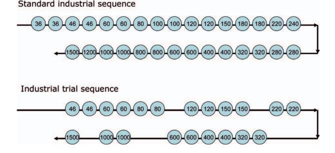
*Figure 5. Abrasive grit sizes used in the sequence of polishing heads in the standard full-scale line (upper diagram) and in the abbreviated sequence used in the industrial trials (lower diagram).*
