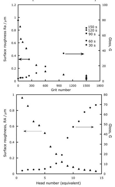
Figure 4. Evolution of surface roughness and gloss of the tile surface as a function of grit number (mesh size) for the abbreviated sequence of polishing steps (as described in the text) in the laboratory-scale rig.
