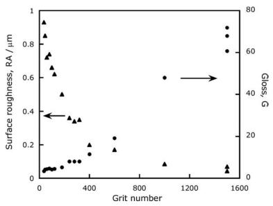
Figure 2. Evolution of surface roughness and gloss of the tile surface as a function of grit number (mesh size) for the full sequence of polishing steps (as described in the text) in the laboratory-scale rig.
