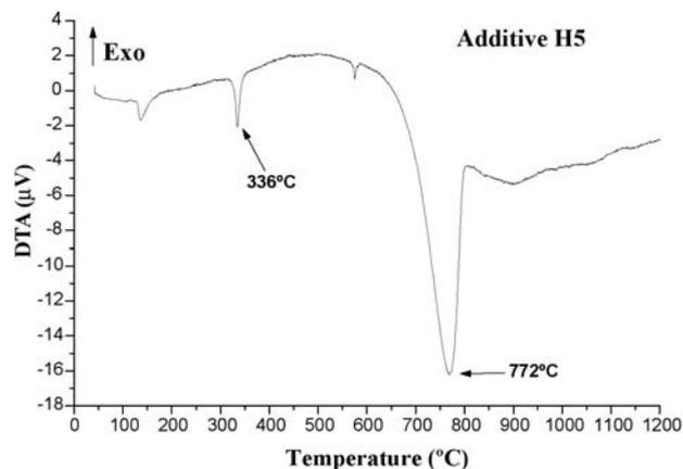
Figure 4. Differential thermal analysis of H5 additive.
