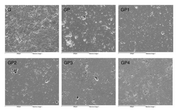
Figure 3. SEM micrographs of as-fired G, polished (GP), polished and treated with con fluoro-carbon resins (GP1), silicon resin in non-aqueous medium (GP2), silicon resin in aqueous medium (GP3),
