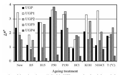
Figure 4. Comparison of the stain resistance ( $\Delta a^*$ ) of the UGP processed surfaces before and after the ageing treatments.
