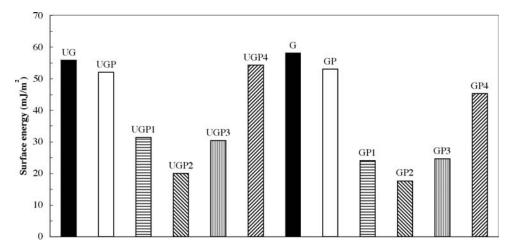
Figure 1. Surface energy of as-fired (UG and G), polished (UGP and GP) tiles, polished and treated with con fluoro-carbon resin (UGP1 and GP1), silicon resin in non-aqueous medium (UGP2 and GP2), silicon resin in aqueous medium (UGP3 and GP3), UV thermo-hardened resin (UGP4 and GP4) tiles.
