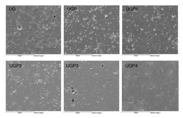
Figure 2. SEM micrographs of as-fired UG, polished (UGP), polished and treated with fluoro-carbon resins (UGP1), silicon resin in non-aqueous medium (UGP2), silicon resin in aqueous medium (UGP3),
