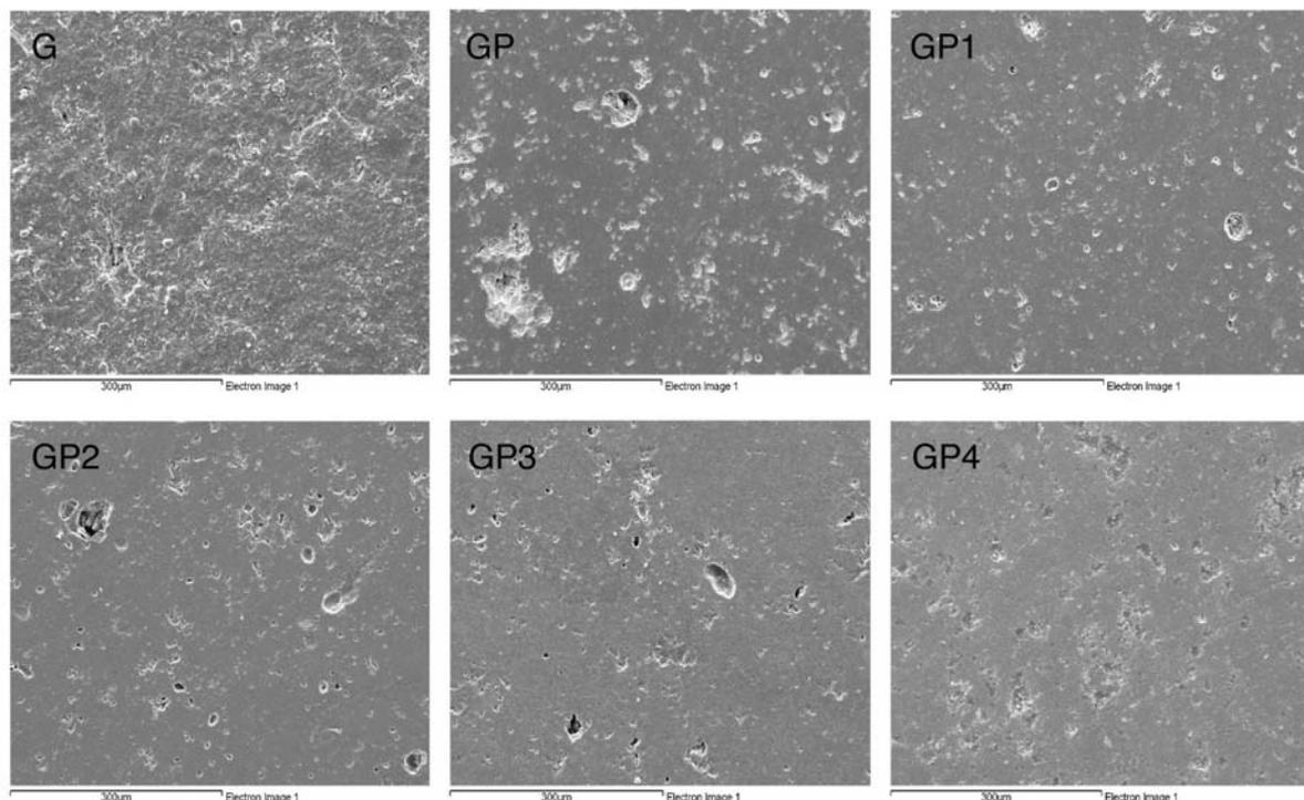
Figure 3. SEM micrographs of as-fired G, polished (GP), polished and treated with con fluoro-carbon resins (GP1), silicon resin in non-aqueous medium (GP2), silicon resin in aqueous medium (GP3), UV thermo-hardened resin (GP4) tiles
