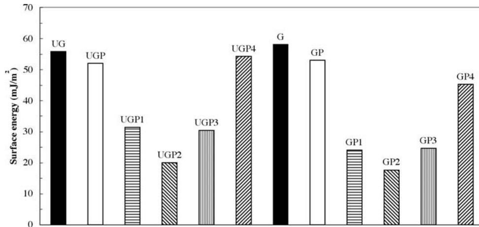
Figure 1. Surface energy of as-fired (UG and G), polished (UGP and GP) tiles, polished and treated with con fluoro-carbon resin (UGP1 and GP1), silicon resin in non-aqueous medium (UGP2 and GP2), silicon resin in aqueous medium (UGP3 and GP3), UV thermo-hardened resin (UGP4 and GP4) tiles.
