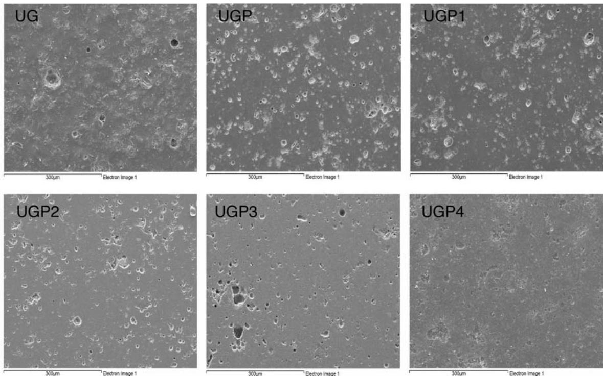
Figure 2. SEM micrographs of as-fired UG, polished (UGP), polished and treated with fluoro-carbon resins (UGP1), silicon resin in non-aqueous medium (UGP2), silicon resin in aqueous medium (UGP3), UV thermo-hardened resins (UGP4) tiles.
