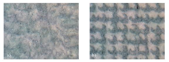
Figure 5. Digital images of blue pigment dots for 80% greyscale with different ink viscosities, a) 16sec and b) 20sec.
