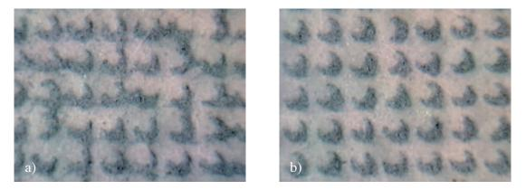
*Figure 1. Digital images of blue pigment dots for 65% greyscale with different production line speeds, a) 15m/min. and b) 53m/min.*
