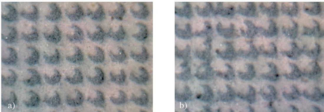
Figure 3. Digital images of blue pigment dots for 65% greyscale with different tile's temperatures, a) 34°C and b) 70°C.
