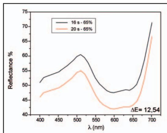
Figure 6. Spectral reflectance of glazed tiles from Figure 5.
