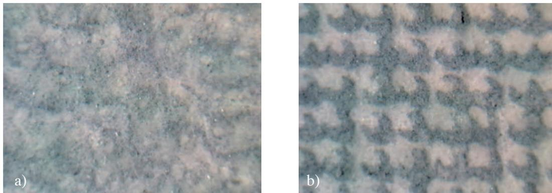
Figure 5. Digital images of blue pigment dots for 80% greyscale with different ink viscosities, a) 16sec and b) 20sec.
