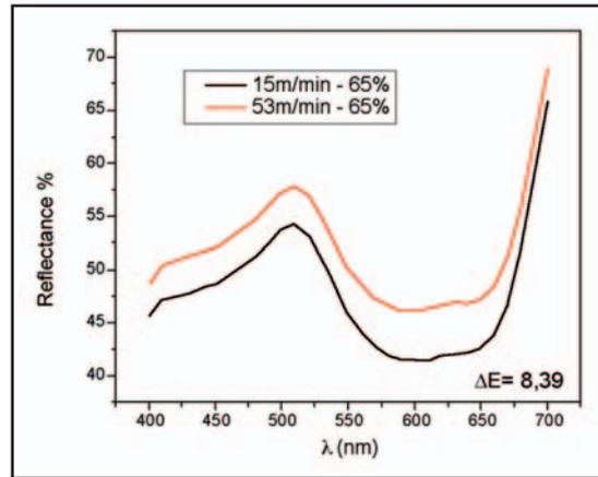
Figure 2. Spectral reflectance of glazed tiles from Figure 1.
