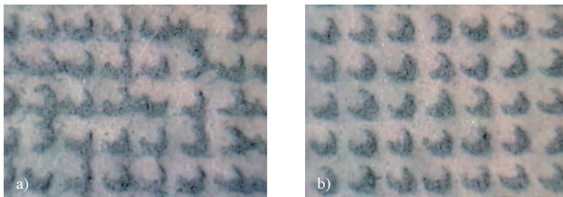
Figure 1. Digital images of blue pigment dots for 65% greyscale with different production line speeds, a) 15m/min. and b) 53m/min.
