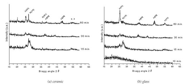
Figure 3 – XRD patterns of  $TiO_2$  thin film by Sputter deposition for 10min, 15min, 30min e 60min onto ceramic (a) and glass (b).
