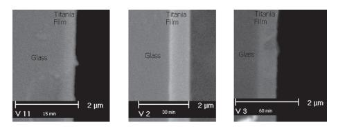
Figure 2. Transversal micrograph of TiO, thin films deposited for 15min, 30min and 60min onto glass substrate.
