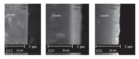
Figure 1. Transversal micrograph of TiO, thin films deposited for 15min, 30min and 60min onto ceramic substrate.
