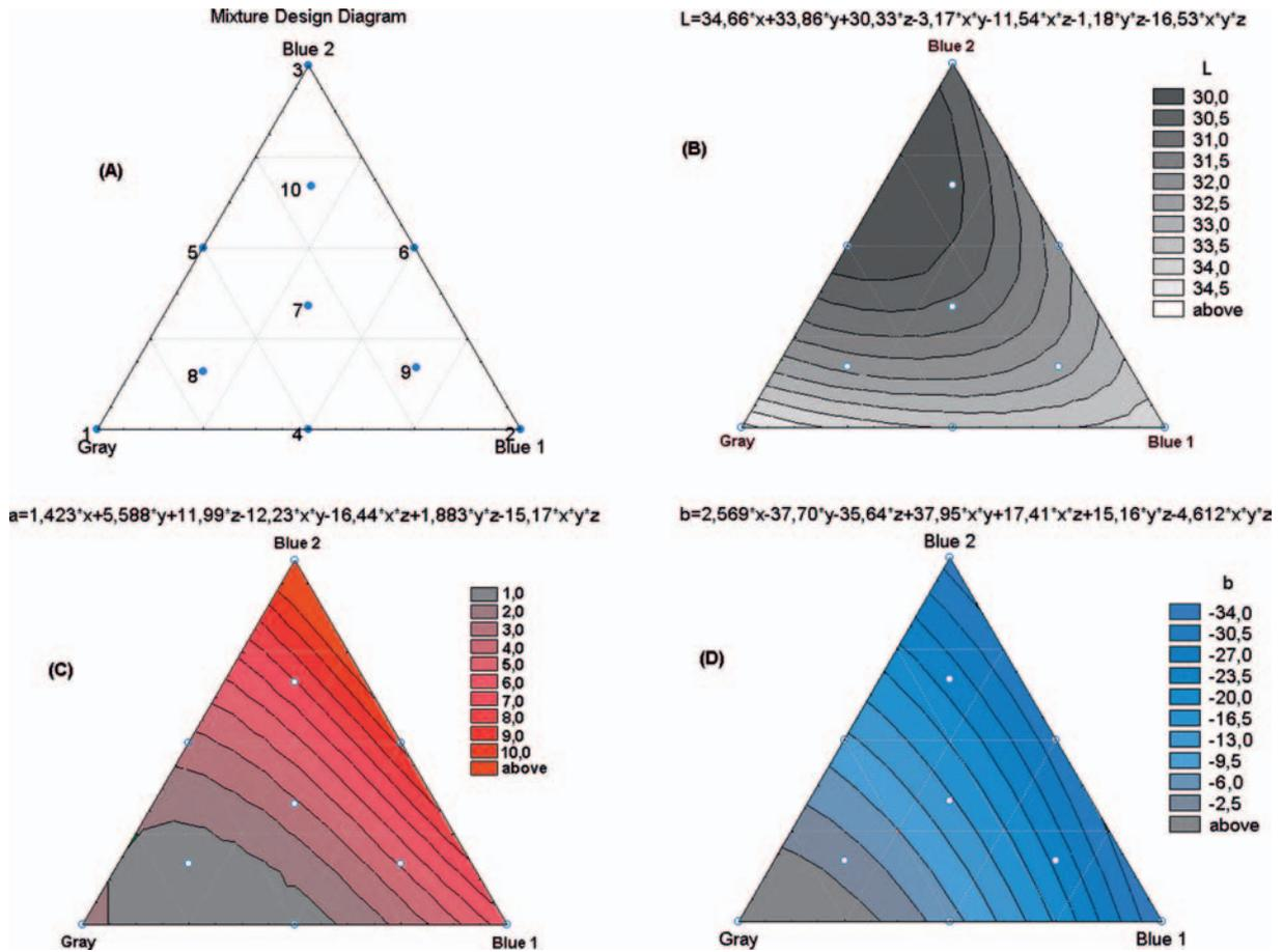
Figure 1. Triaxial diagrams of the studied system: (A) experimental design, and response surfaces for (B)  $L$ , (C)  $a$ , and (D)  $b$ , respectively.
