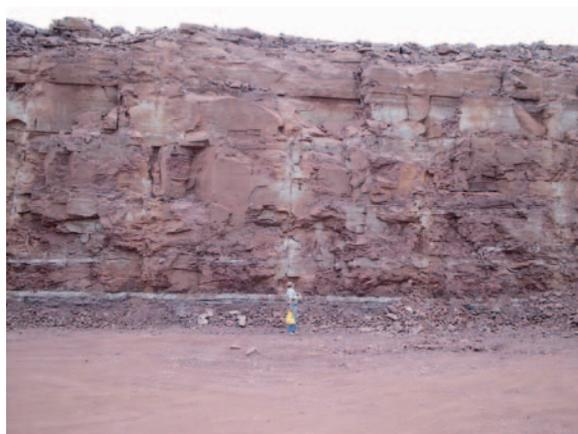
Image 2. General view of a mine in the top of the Corumbataí Formation, made up of chestnut-purple argillite with decimetre interleaves containing a great amount of carbonates.
