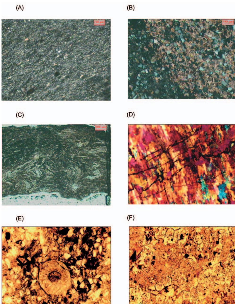
*Image 1. Micrographs of sheets of the Corumbataí Formation, showing, in decreasing order of occurrence, the mineralogical composition: (a) Illitic matrix; (b) Arcabuz consisting of quartz and feldspars with carbonate cement; (c) Neo-formed feldspar occurrence; (d) Quartz vein; (e) Fossil fragment; (f) Analcime.*
