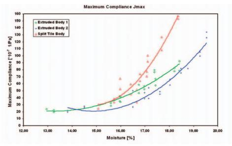
*Figure 3. Comparison of the maximum compliance for three different production bodies, derived from the rheological creep test.*
