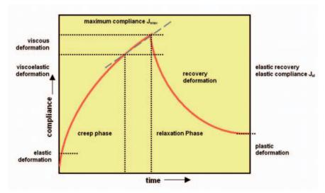
Figure 2. The creep compliance test
