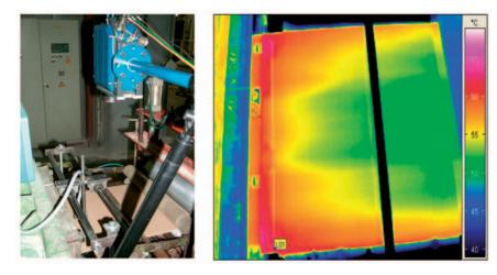
Figure 1. The experimental setup for the thermography measurement and the measured temperature profile
