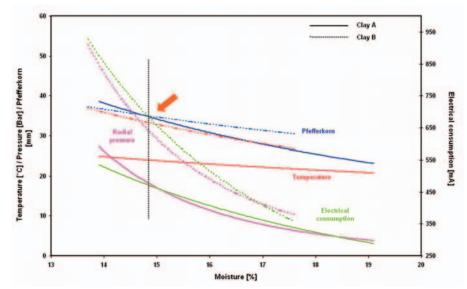
Figure 5. Comparison of two different clay mixtures used in bodies for extruded tiles using the laboratory press.
