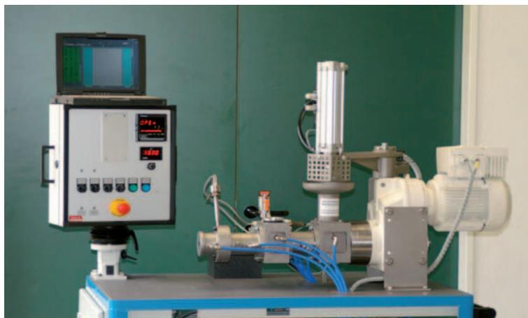
Figure 4. The vacuum laboratory press as used in the project
