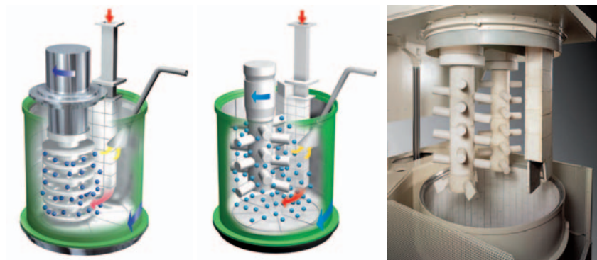
Figure 1. Configuration of the MaxxMill® - disk type tool (left), bar type tool (middle), opened MaxxMill® MM5 with 2 eccentrically positioned bar agitators (right)
