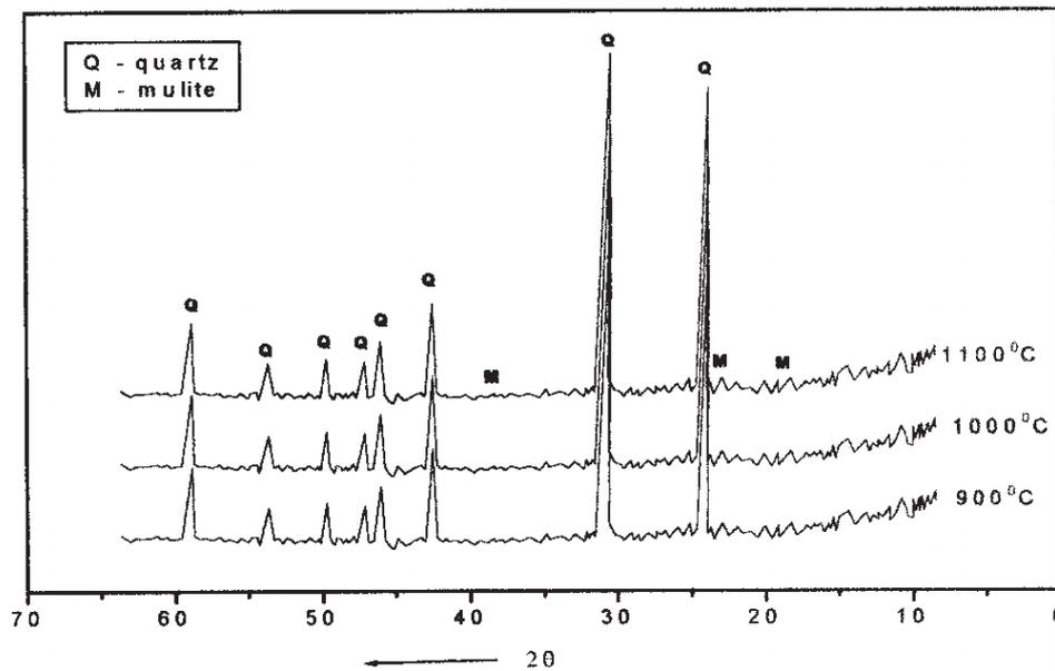
Figure 4. X-ray data of the clay sandstone thermally treated at 900, 1000 and 1100°C.
