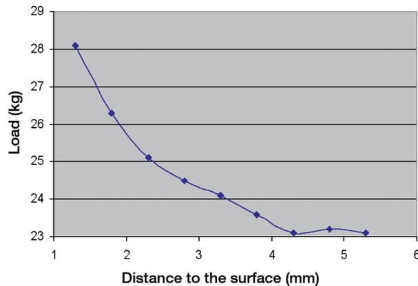
Figure 1. Bending test breaking load versus distances of the fibres to the surface.
