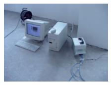
Figure 2. Temperature data logger, model SCX1300 of National Instruments
