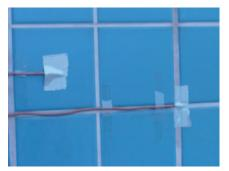
Figure 1. Position of the thermocouples on the building facade.
