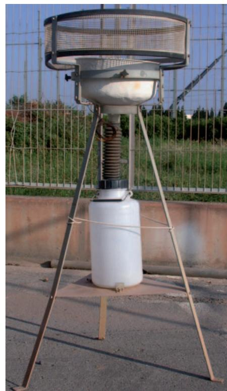
Figure 1. Settleable particulate sampler.
