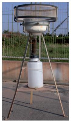
Figure 1. Settleable particulate sampler.
