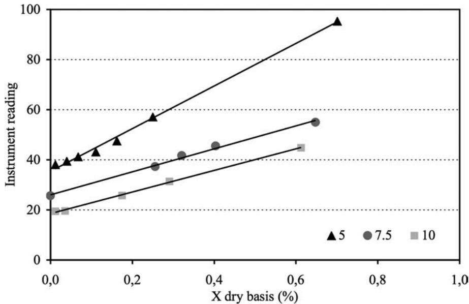
Figure 3. Effect of instrument–tile distance on the reading
