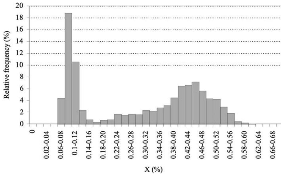
Figure 13. Histogram of overall tile moistures after a long shutdown
