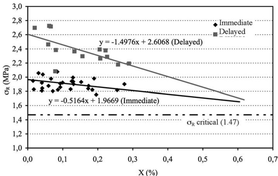
Figure 14. Comparison of mechanical strength in immediate and delayed measurement
