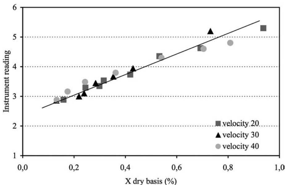
Figure 4. Effect of tile passage velocity on the instrument reading
