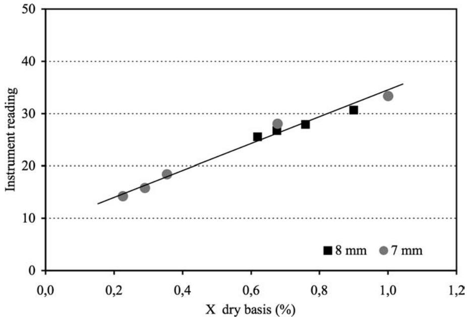
Figure 6. Effect of the variation of tile thickness on the instrument reading
