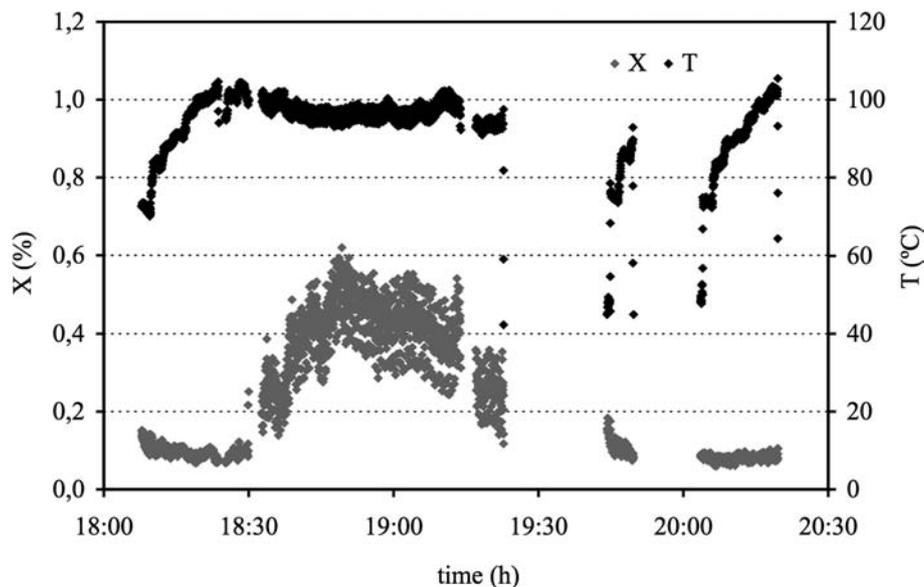
Figure 12. Tile moisture and temperature during operation with long stoppages
