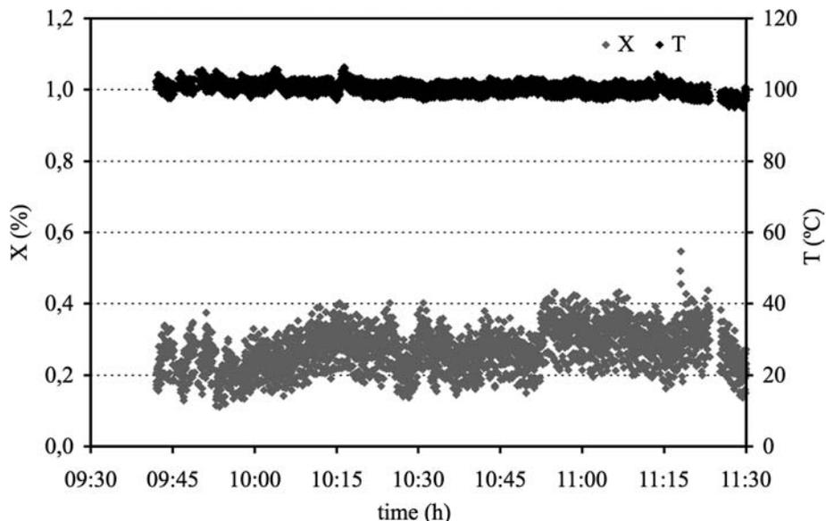
Figure 10. Tile moisture and temperature values during steady dryer operation
