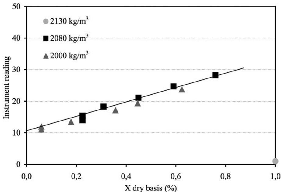
Figure 7. Effect of tile bulk density on the instrument reading
