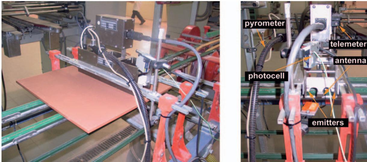
Figure 2. General view of the radio frequency instrument measuring tile moisture content at ITC
