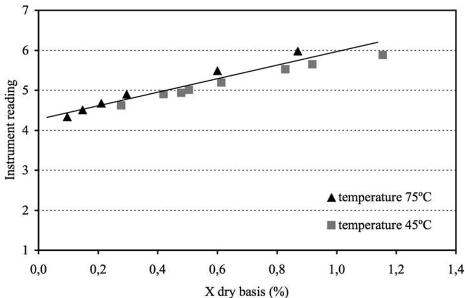
Figure 5. Effect of tile temperature on the instrument reading
