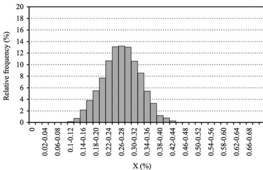
Figure 11. Histogram of tile residual moisture during steady operation
