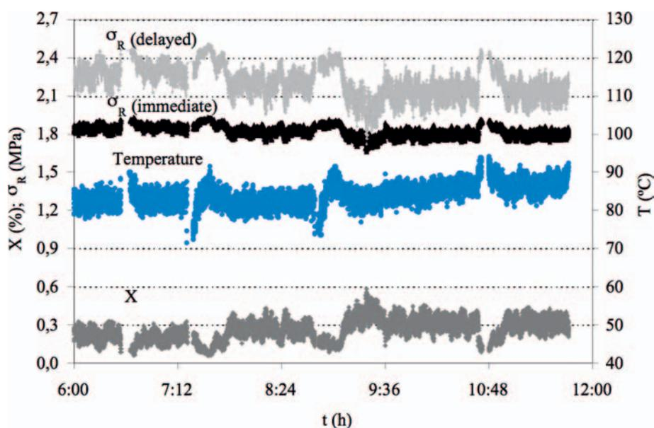
Figure 15. Values of  $\sigma_R$  obtained by calibration together with the  $X$  and  $T$  of the tiles at the dryer exit
