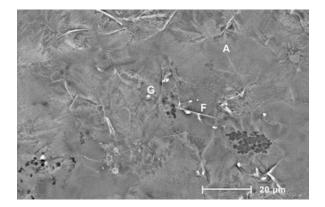
*Figure 8. Surface of the piece at 1100°C-0'.Normal cooling.*
