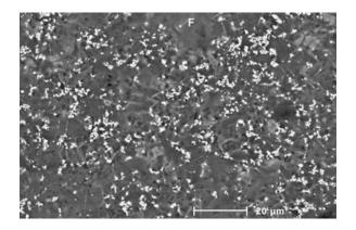
Figure 7. Surface of the piece at 1000°C-0'. Normal cooling.
