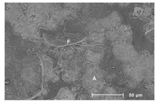
Figure 9. Surface of the piece 1190 °C–0'. Normal cooling.
