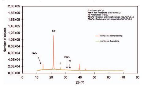
Figure A3. Comparison of cooling cycles at 1190°C
