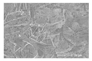
Normal cooling. Figure 5. Tile surface 1190  $^{\circ}\mathrm{C}-8'.$
