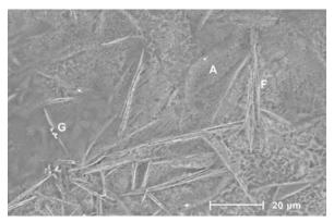
Quenching. Figure 6. Tile surface 1190 °C – 8'.
