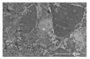
*Figure 10. Surface of the piece 1220 °C–0'. Normal cooling.*
