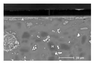
Figure 4. Observation of the (bevelled) cross-section of the glaze layer on the industrial tile.
