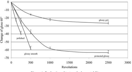
Figure 6. Evaluation of test method repeatability
