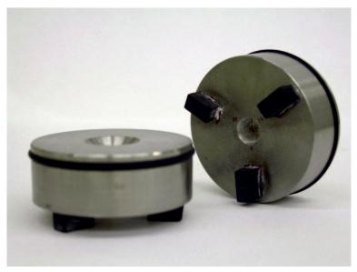
Figure 1. Abrasion device
