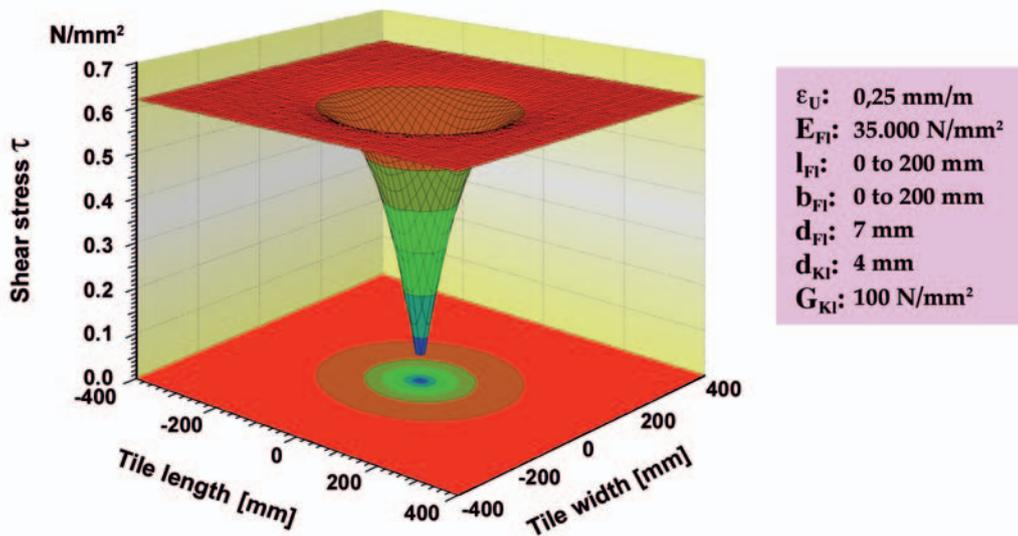
Figure 8. Maximum shear stress in the corners of the tile as a function of tile edge length
