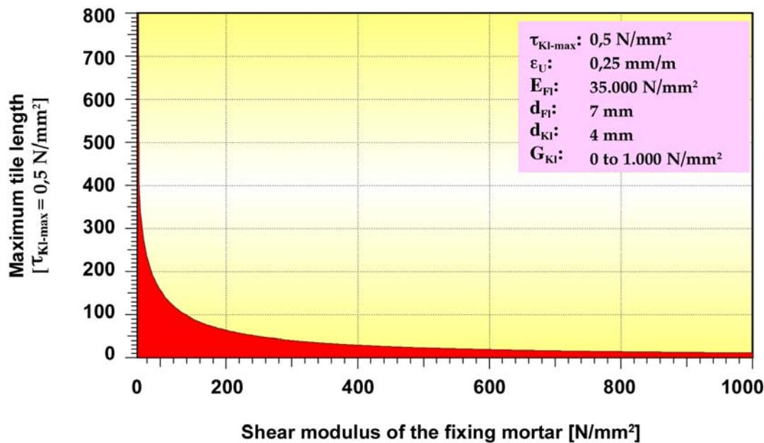
Figure 9. Maximum tile size as a function of adhesive shear modulus, when the maximum shear stress shall not exceed 0.5 N/mm<sup>2</sup>
