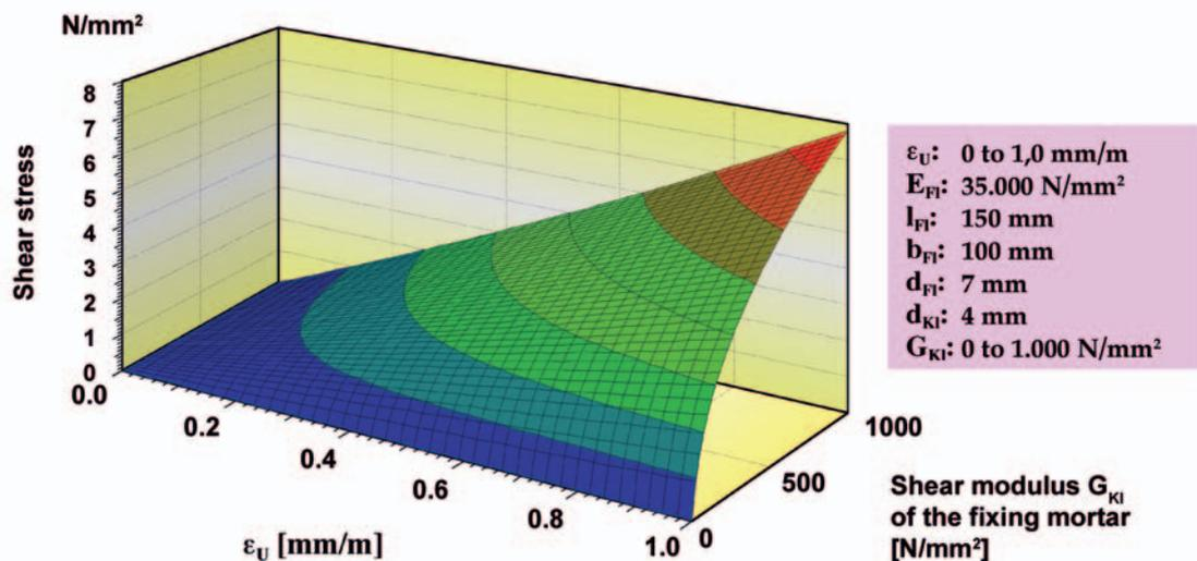
Figure 7. Influence of base deformation and shear modulus of the cementitious adhesive on the maximum shear stress in the corners of the tile
