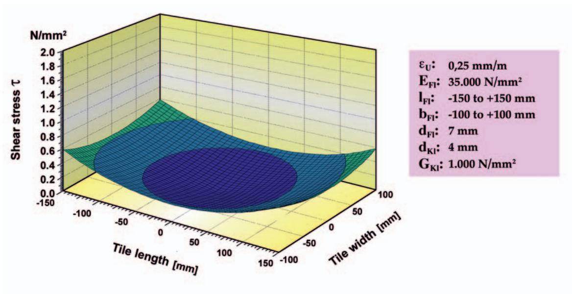
Figure 6. Distribution of the shear stress for a flexible fixing mortar
