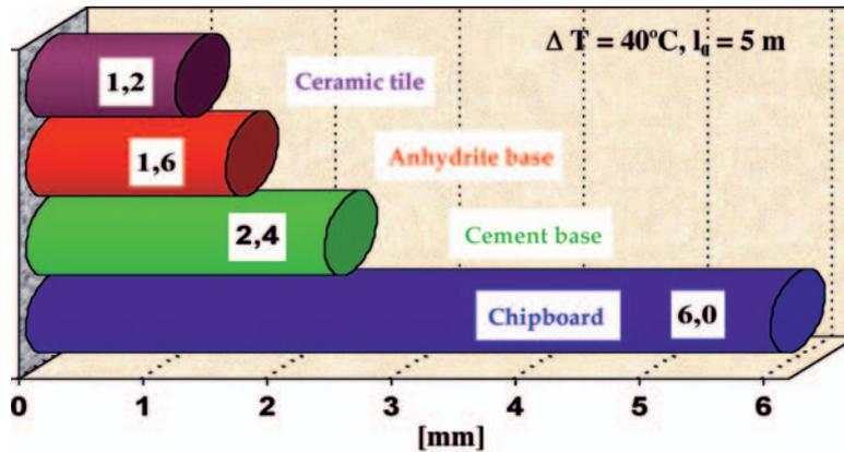
Figure 2. Absolute longitudinal expansion of a terrace tiling
