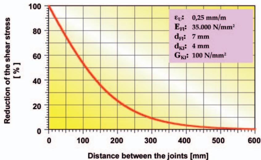
Figure 10. Reduction of maximum shear stress by the joints in the ceramic tiling
