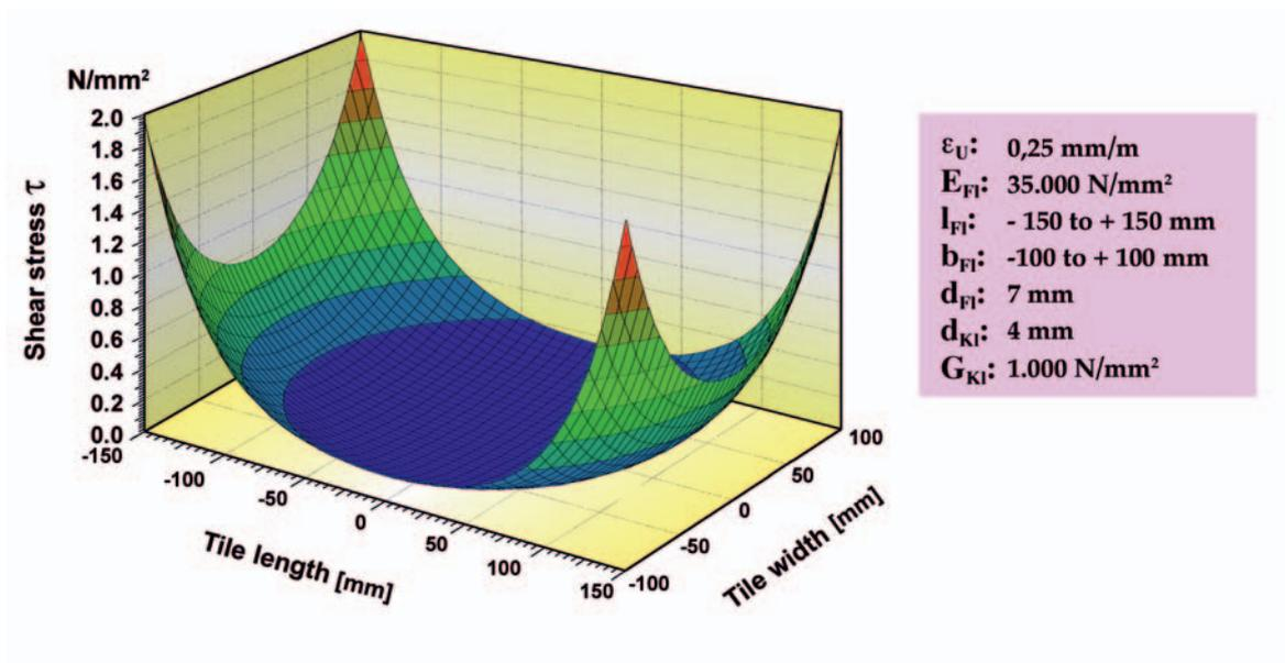
Figure 5. Radial distribution of the shear stress for a rigid fixing mortar
