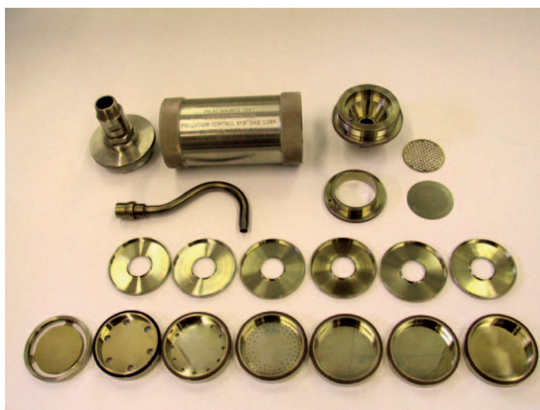
Figure 2. Detail of the disassembled MARK III cascade impactor
