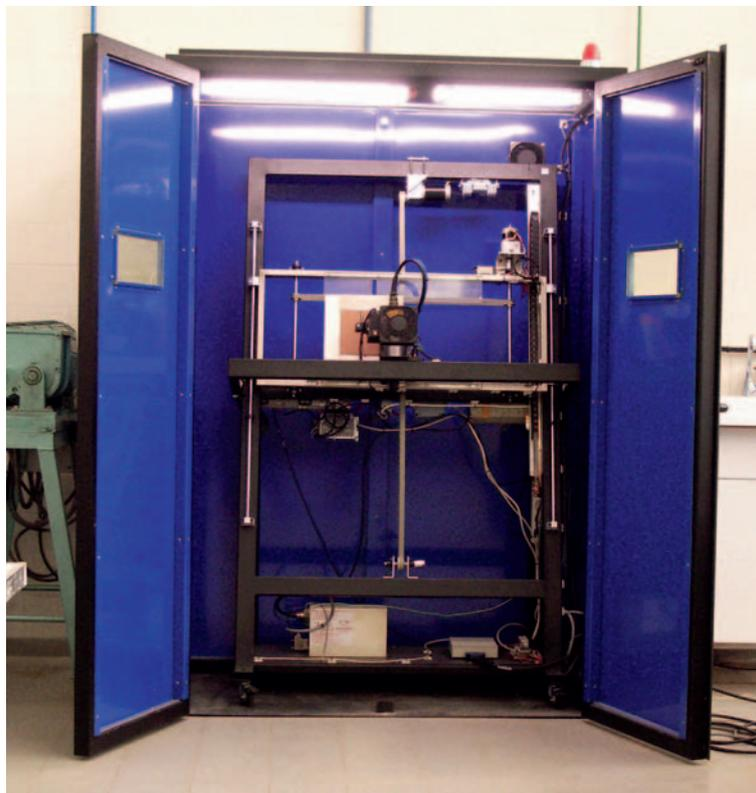
Figure 2. Prototype for bulk density measurement by X-ray absorption.
