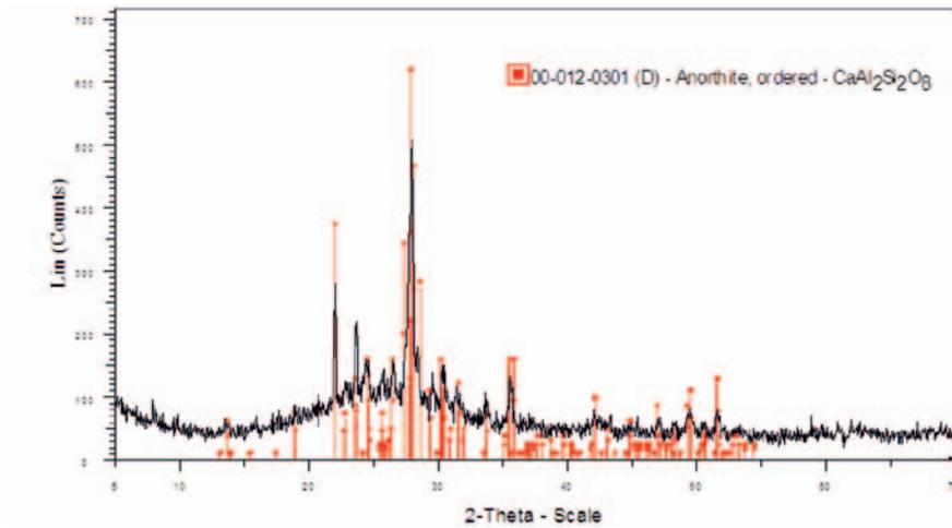
Figure 7. XRD spectrum of the fired MT glaze.
