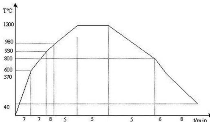
Figure 3. Firing cycle used in porcelain tile production.
