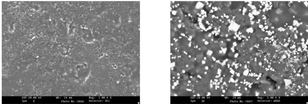
Figure 12. Micrograph (5000x) of the tile surface coated with MO+AD.
