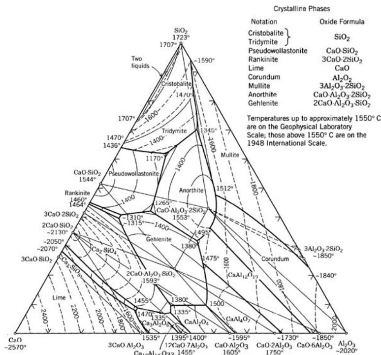
Figure 1. Phase diagram of the system  $\text{CaO-Al}_2\text{O}_3\text{-SiO}_2$ <sup>[8]</sup>.
