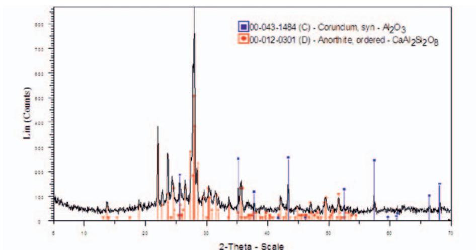
Figure 9. XRD spectrum of the fired MT+AD glaze.
