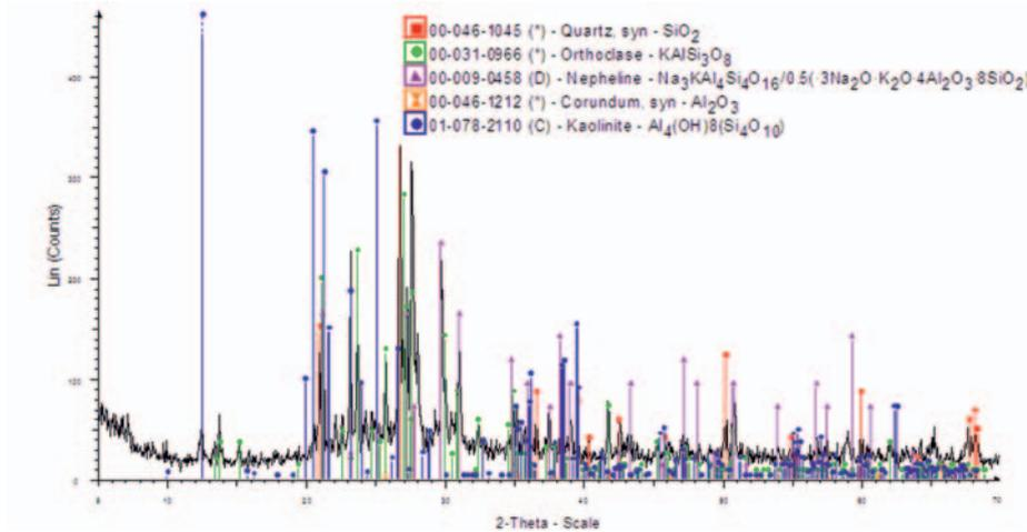
Figure 4. XRD spectrum of the unfired MT glaze.
