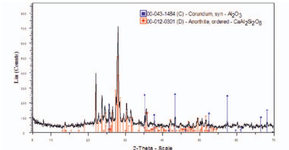
Figure 10. XRD spectrum of the fired MO+AD glaze.
