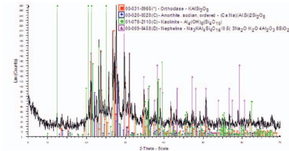
Figure 5. XRD spectrum of the unfired MO glaze.
