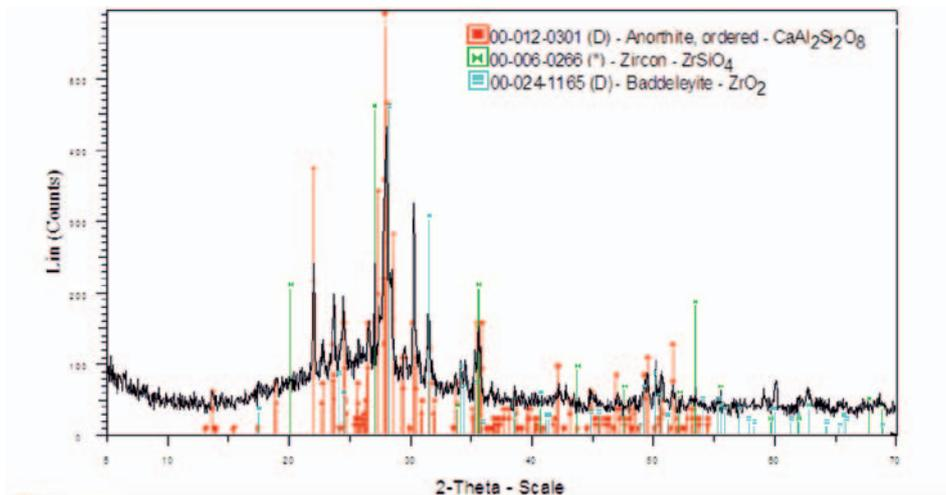
Figure 8. XRD spectrum of the fired MO glaze.
