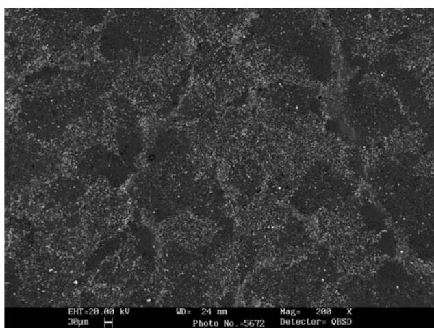
Figure 11. Micrograph (200x) of the tile surface coated with MO+AD.
