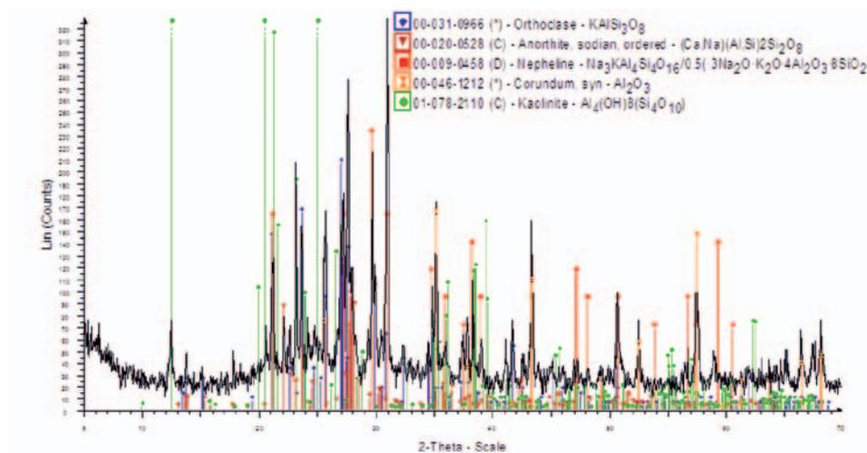
Figure 6. XRD spectrum of the unfired AD glaze.
