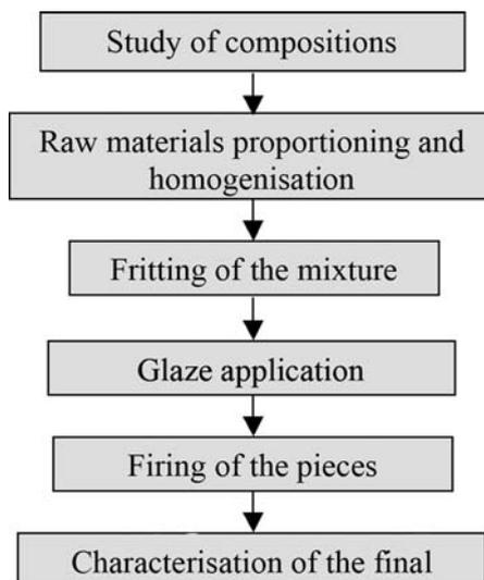
Figure 2. Flow chart followed in developing the glass-ceramic glazes
