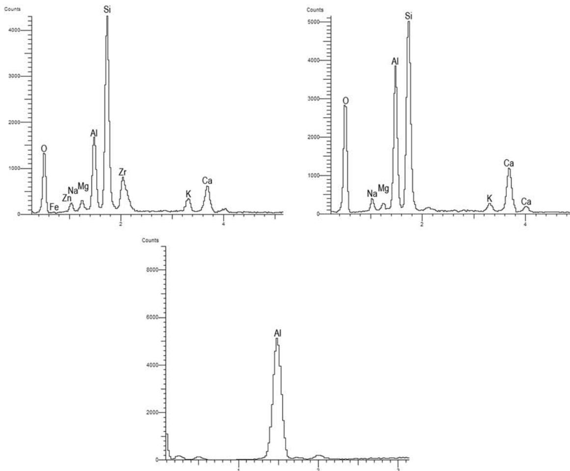
Figure 13. EDX microanalyses of the tile surface coated with MO+AD
