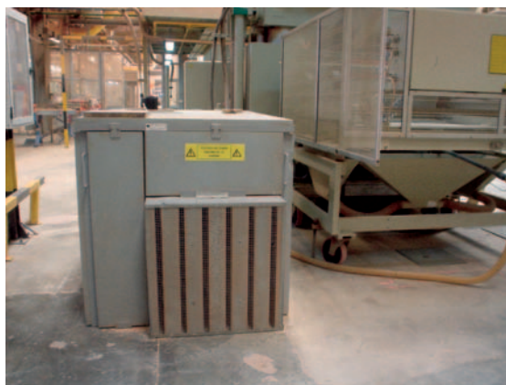
Soundproofing of the hydraulic manifold of a clay press. The envelope is fitted with a fan to dissipate the heat inside.
