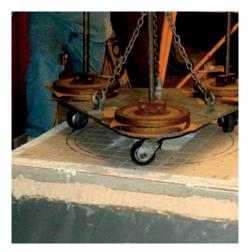
Figure 1. Robinson-Type Floor Tester
