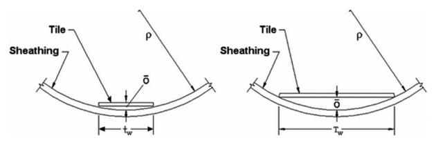
Figure 5. Sensitivity to Curvature Increases with Tile Format
