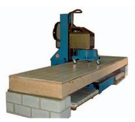
Figure 3a. Universal Floor Tester Full-Scale Assembly
