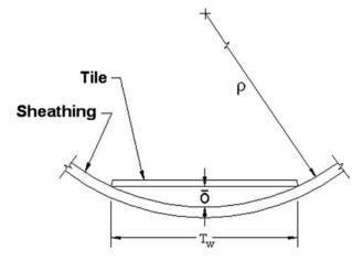
Figure 4. Exaggerated View of Curvature of Wood Subfloor beneath Tile Covering
