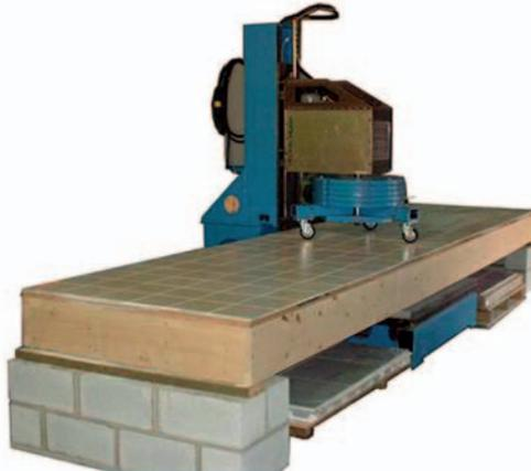
Figure 3a. Universal Floor Tester Full-Scale Assembly
