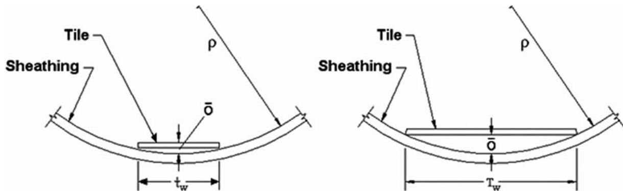
Figure 5. Sensitivity to Curvature Increases with Tile Format
