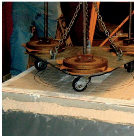
*Figure 1. Robinson-Type Floor Tester*
