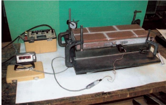
Figure 2. System Crack Resistance Tester
