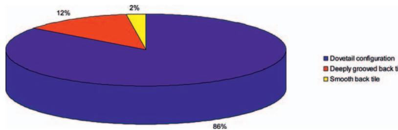
Figure 6 – Configuration of back side of ceramic tiles.
