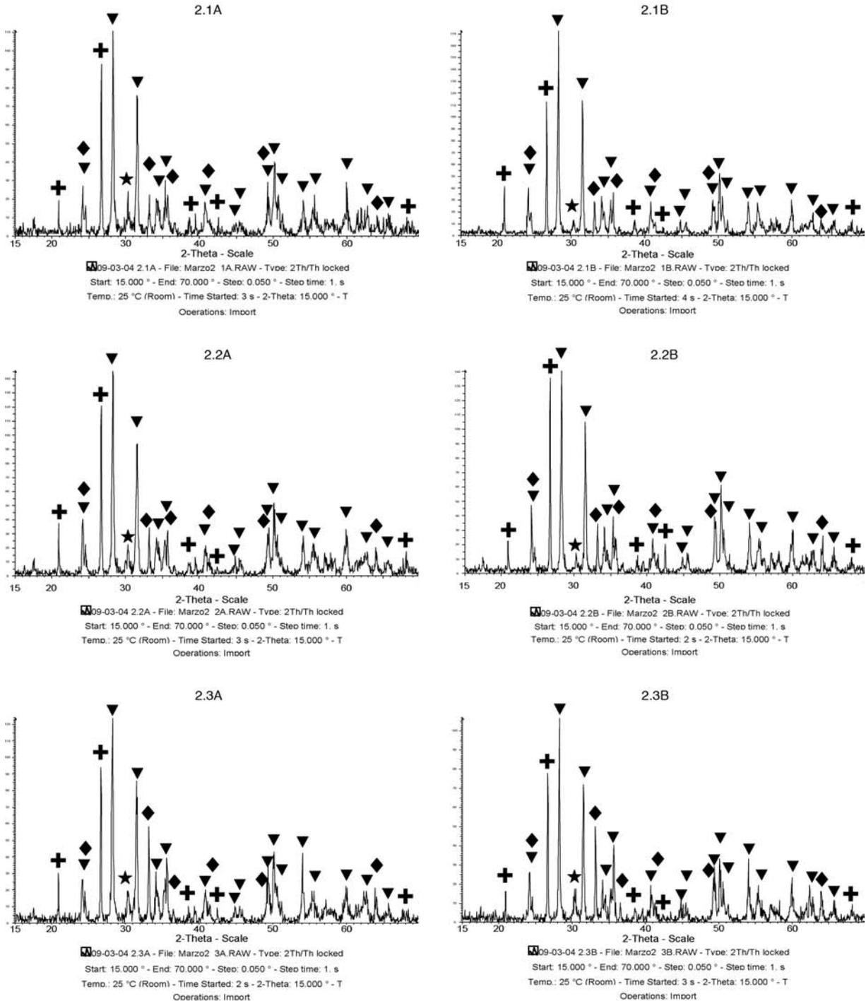
▼ Baddeleyite      + Quartz      ◆ Hematite      ★ Zirconium oxide
