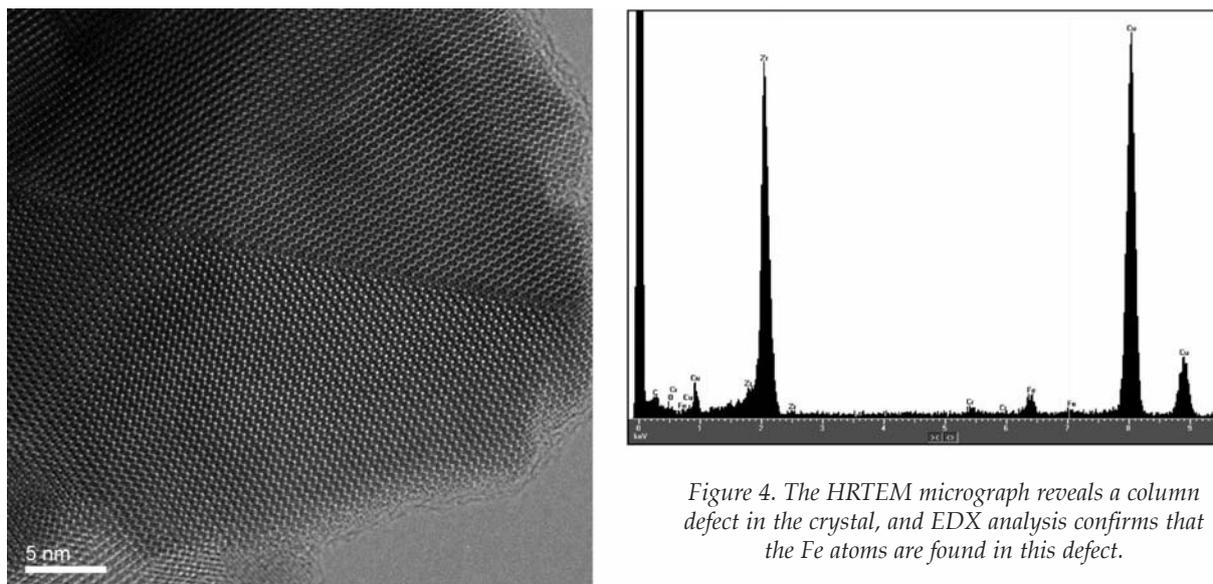
Figure 4. The HRTEM micrograph reveals a column defect in the crystal, and EDX analysis confirms that the Fe atoms are found in this defect.
