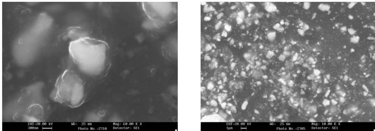
Figure 3. SEM of sample 3.3 (10% Fe) at a magnification of 60,000x and at 10,000x
