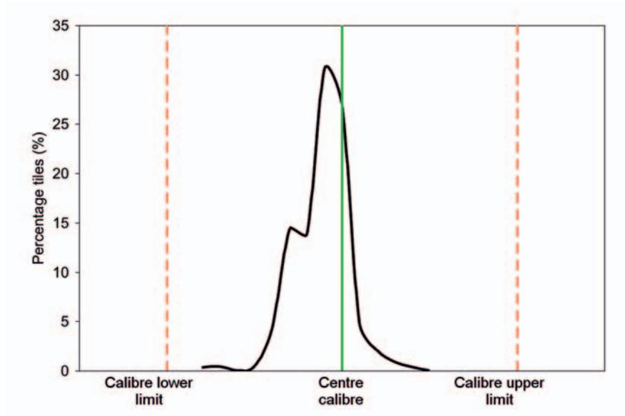
Figure 20. Classification by sizes of the tiles made with the activated automatic control system (3000 m<sup>2</sup>, of nominal size 45 x 67.5 cm).
