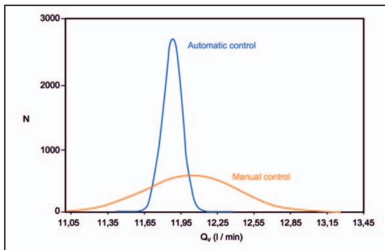
Figure 10. Distribution of glaze volume flow rates with manual and automatic control
