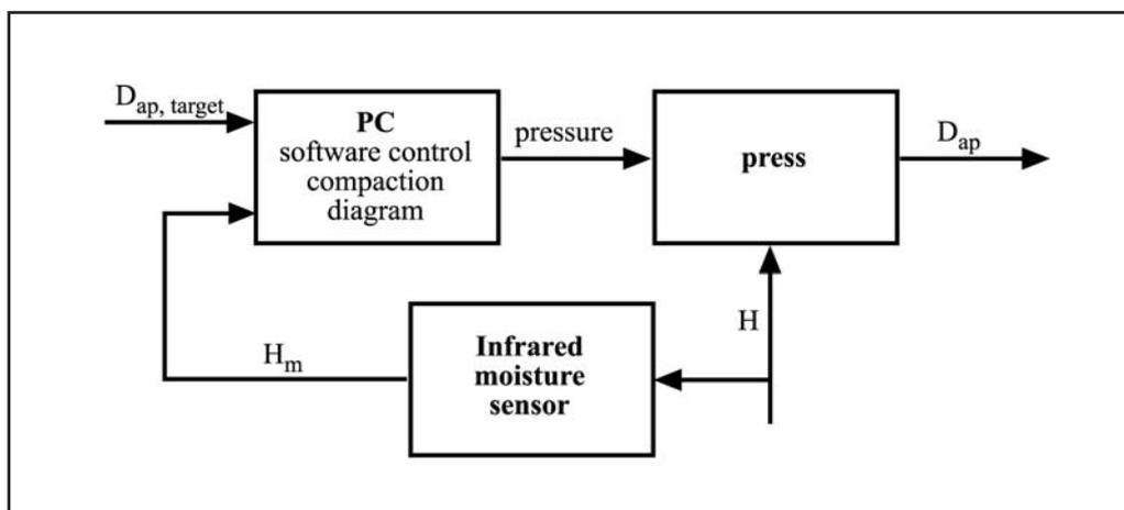
Figure 16 . Block diagram of feedforward control
