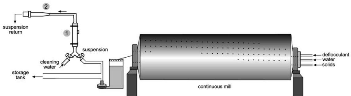
Figure 3. Scheme of the arrangement of the measuring elements in an industrial continuous mill.
