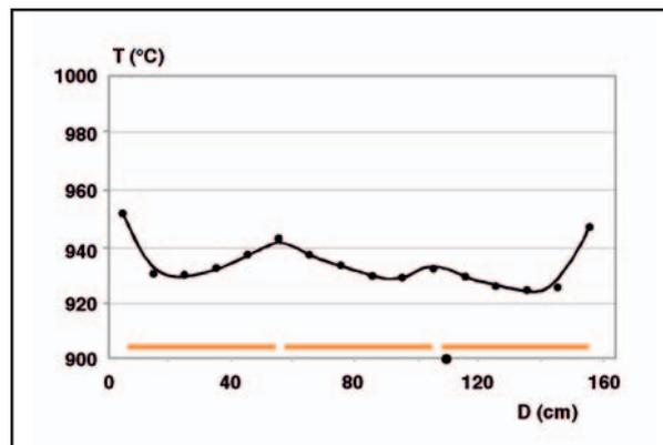
Figure 12. Transverse temperature gradients inside the kiln
