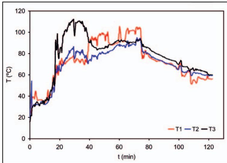
Figure 7. Gas temperature distribution in a vertical dryer during a drying cycle, in different positions
