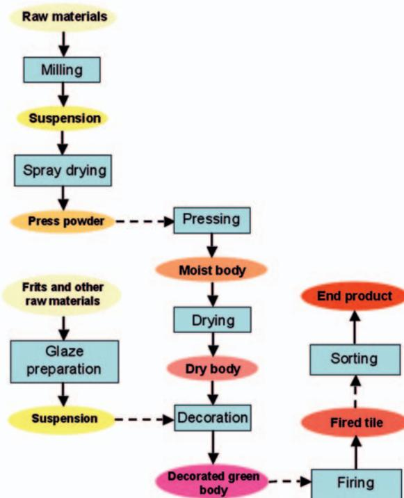
Figure 1. Manufacturing process of pressed and glazed ceramic tiles by single firing, using the wet method.
