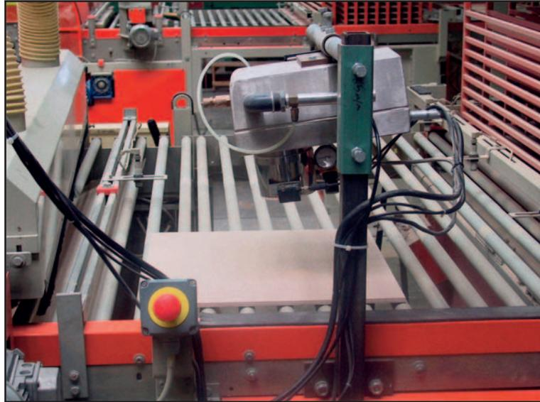
Figure 15. On-line moisture measurement of ejected compacts
