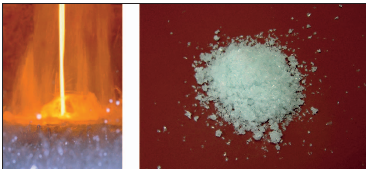
Figure 9. Glassy appearance of ceramic frits after the fusion and fritting stages.
