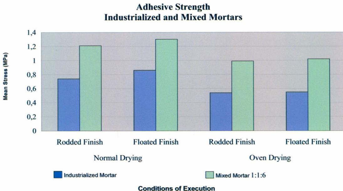
Graph 6. Surface adhesive strength of the tiling with industrialized mortar
