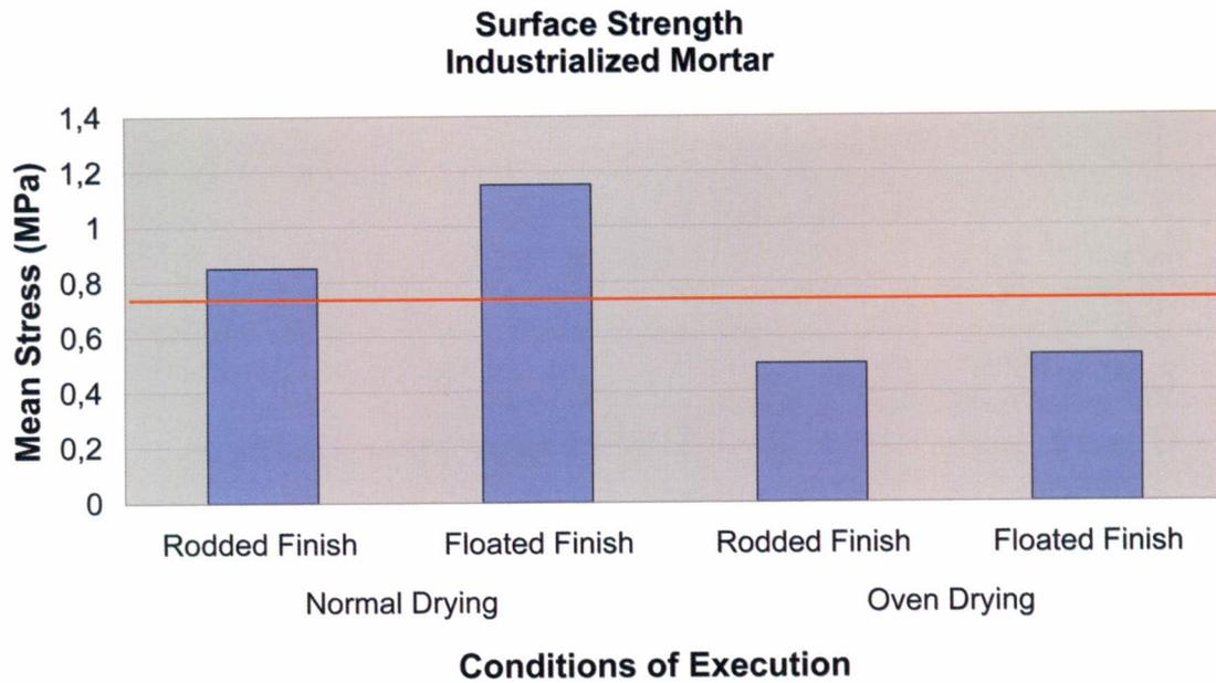
Graph 1. Surface adhesive strength of the tile with industrialized mortar
