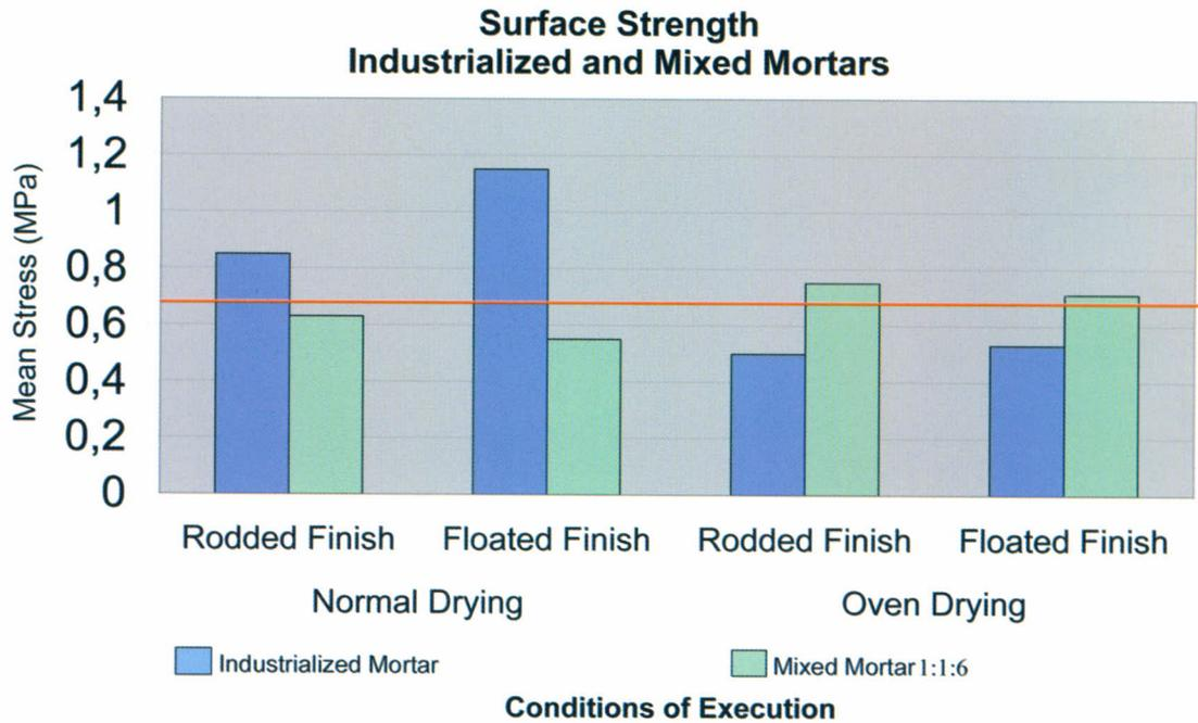
Graph 3. Tiling surface adhesive strength with industrialized and mixed mortar
