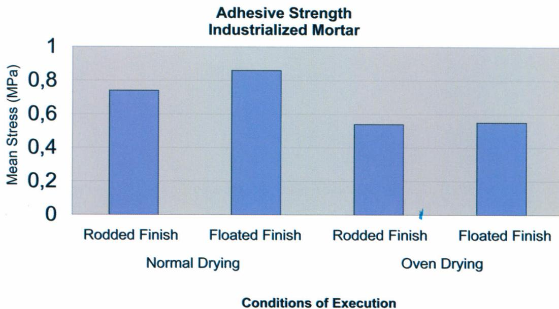
Graph 4. Tiling adhesive strength with industrialized mortar
