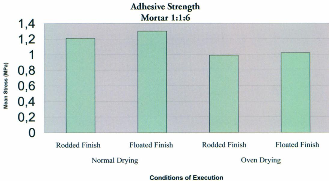
Graph 5. Tiling adhesive strength with industrialized mortar
