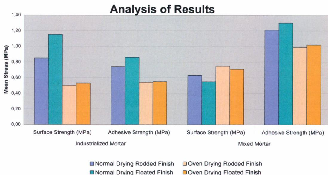
Graph 7. Parge coat surface strength and tiling adhesive strength
