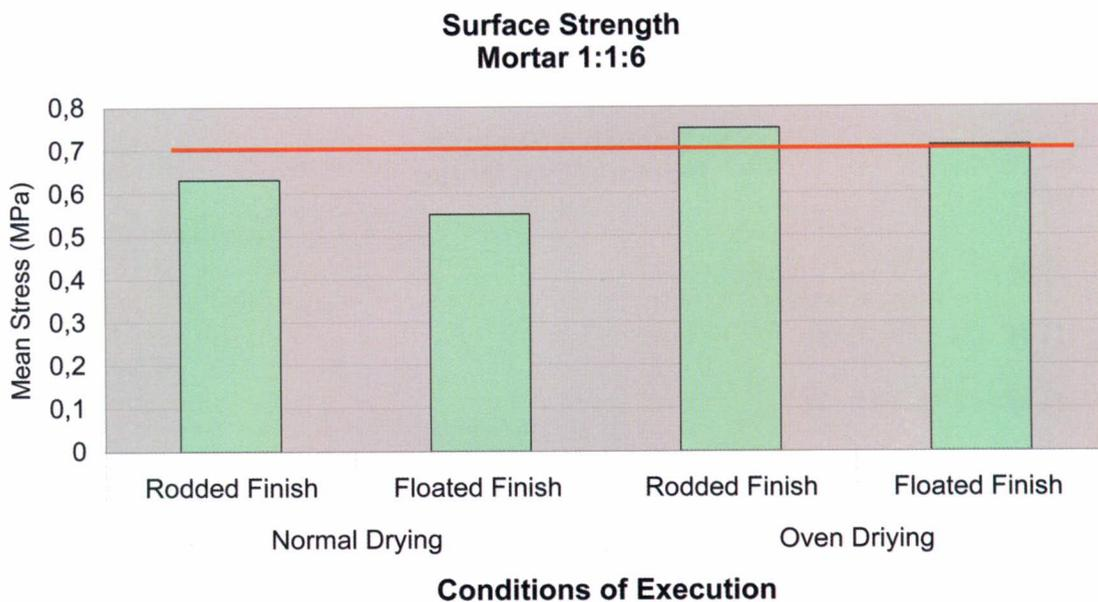
Graphic 2. Surface adhesive strength of the tile with industrialized mortar
