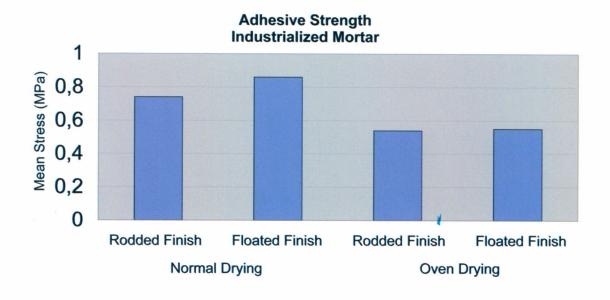
Graph 4. Tiling adhesive strength with industrialized mortar
