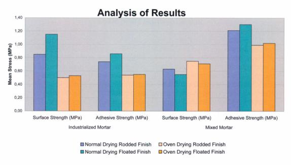
Graph 7. Parge coat surface strength and tiling adhesive strength
