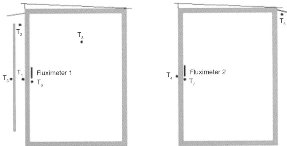
Figure 4. Temperature sensors and fluximeter position in the ventilated facade and the conventional facade, respectively.
