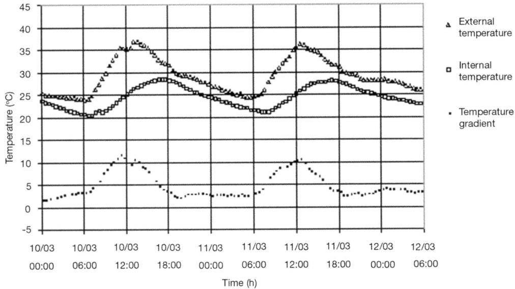
Figure 7. External and internal temperatures in the condition of summer with sunny weather (with ventilation in the air chamber).
