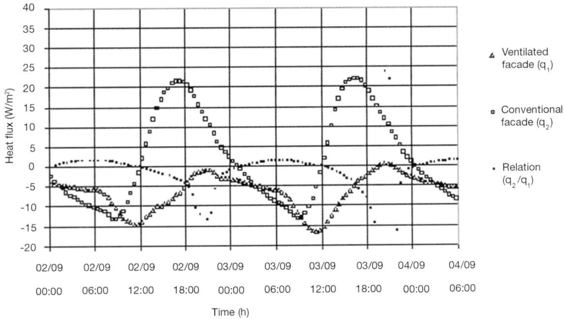
Figure 12. Heat fluxes in the facades (with ventilation in the air chamber) and relation  $q_2/q_1$  in the condition of winter with sunny weather.
