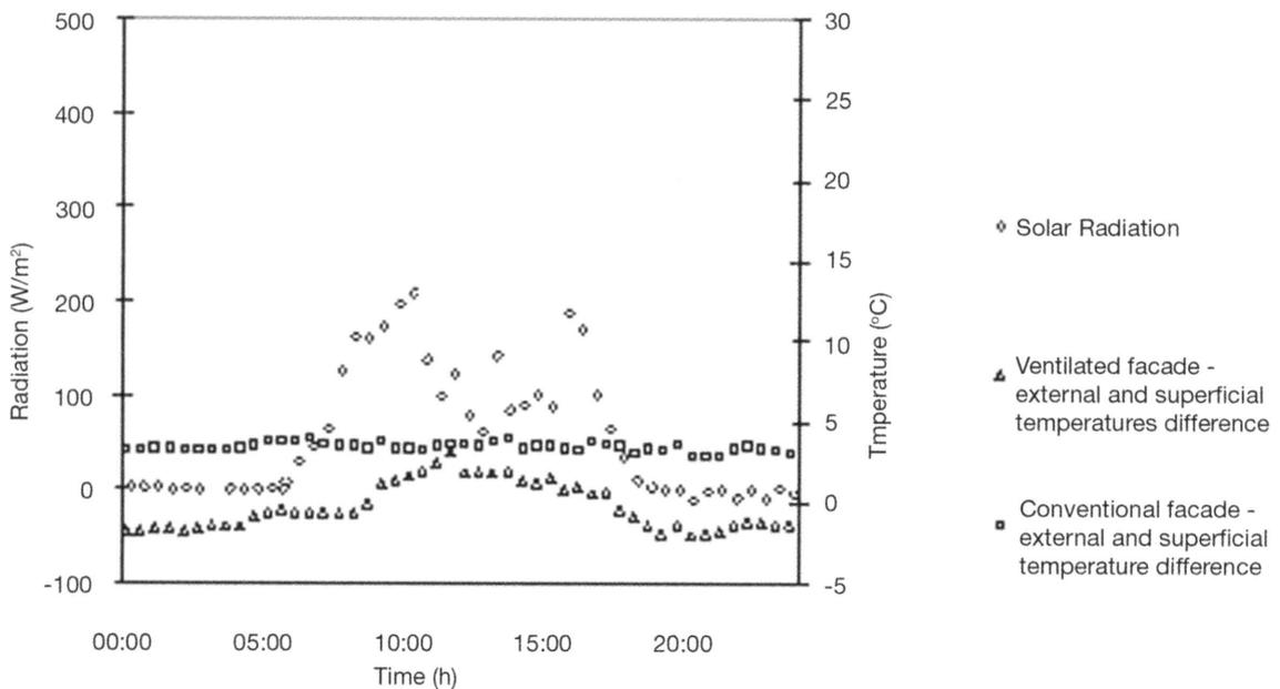
Figure 6. Relation between incident solar radiation values and differences between superficial and external temperatures in characteristic day with cloudy weather.
