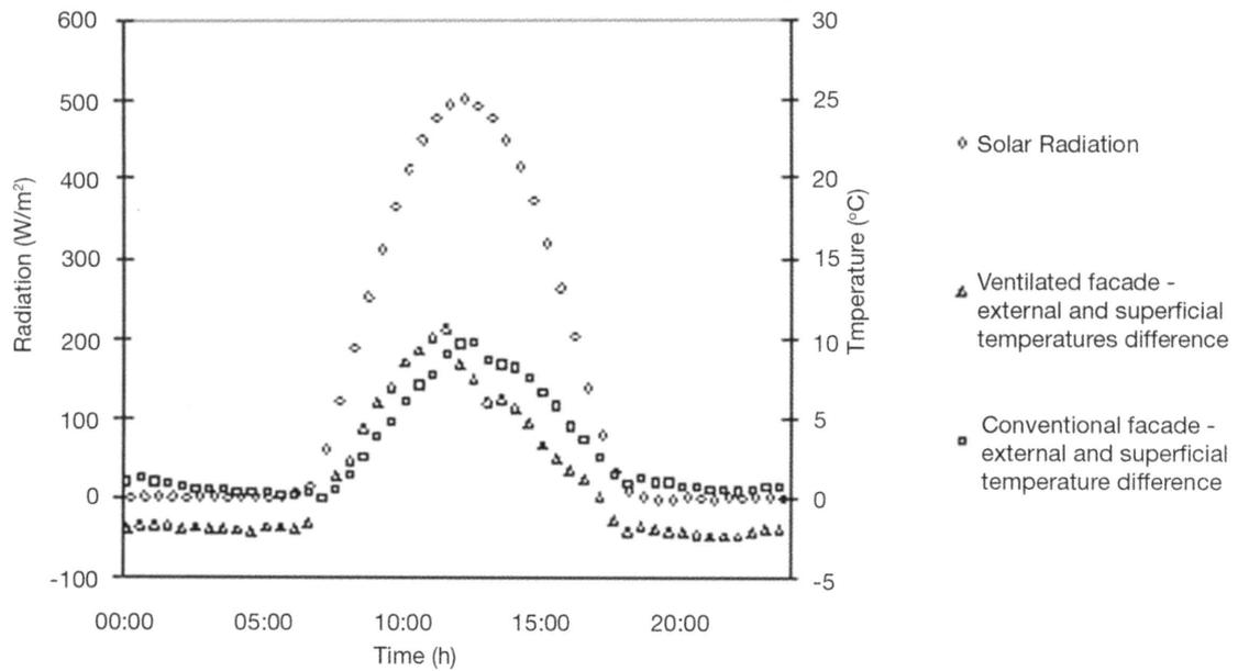
Figure 5. Relation between incident solar radiation values and differences between superficial and external temperatures on a characteristic day with sunny weather for ventilated and conventional facades.
