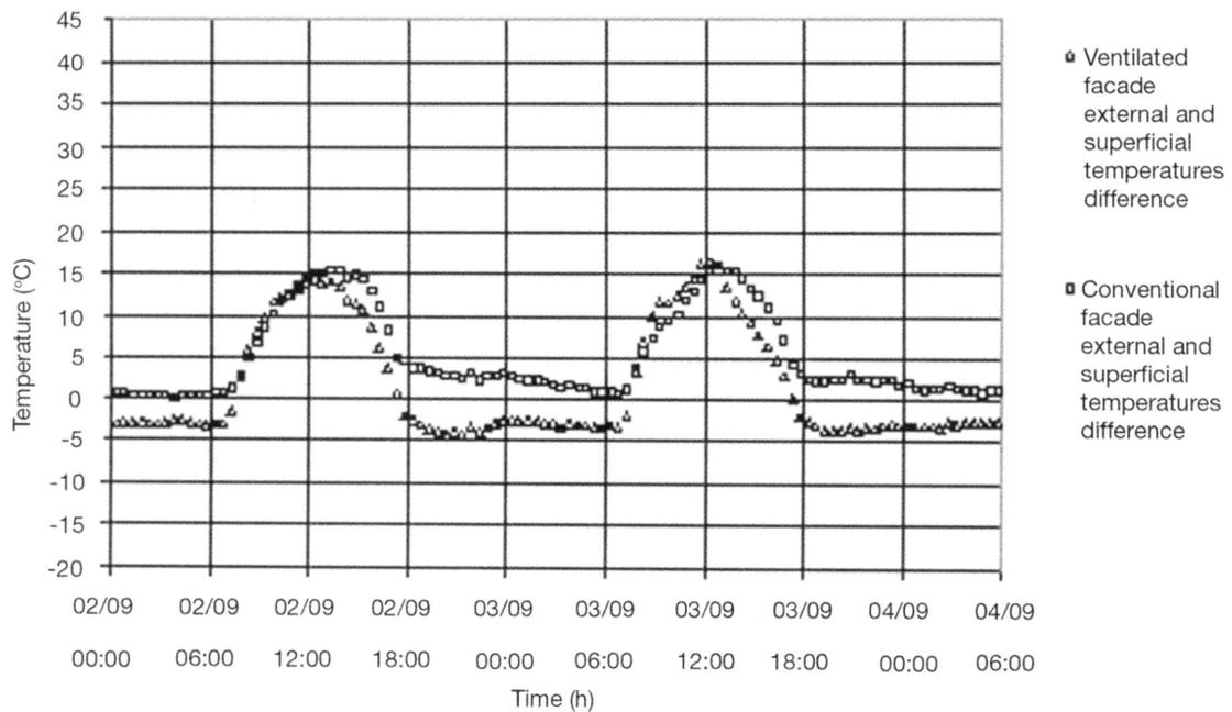
Figure 11. Differences between external superficial temperatures and external ambient temperatures on the analysed days.
