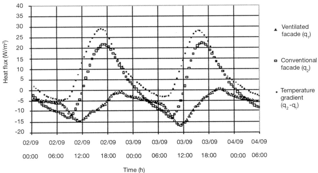
Figure 13. Heat fluxes in the facades (with ventilation in the air chamber) and difference  $q_2 - q_1$  in the condition of winter with sunny weather.
