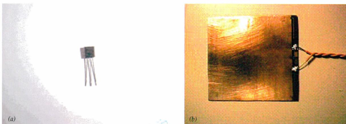
Figure 3. Integrated temperature sensors LM35 - National Semiconductos (a) and "tangential gradient" fluximeter (b).
