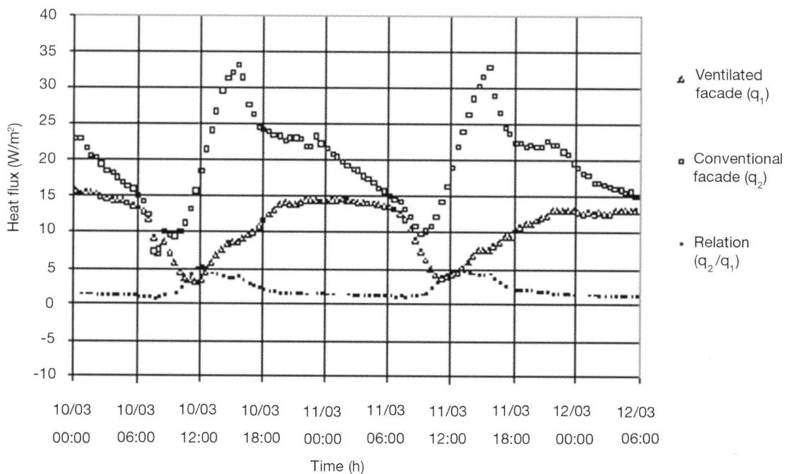
Figure 9. Heat fluxes in the facades (with ventilation in the air chamber) and relation  $q_2/q_1$  in the condition of summer with sunny time.
