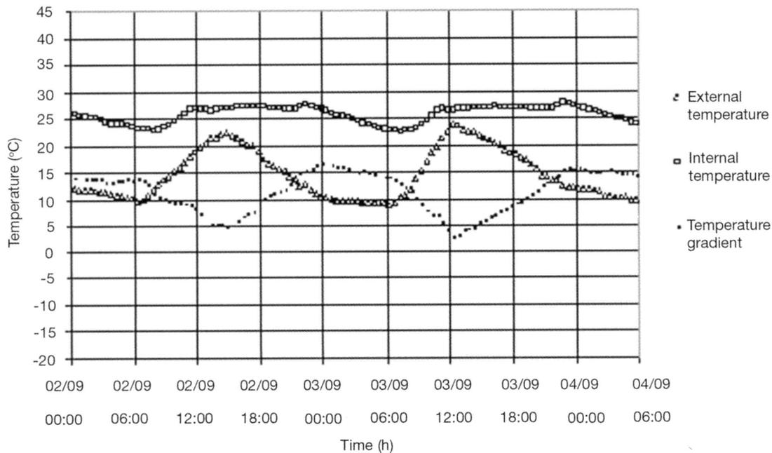
Figure 10. External and internal temperatures in the condition of winter with sunny weather (with ventilation in the air chamber).
