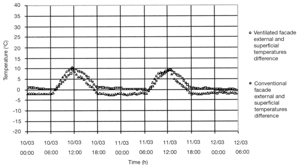
Figure 8. Differences between external superficial temperatures and external ambient temperatures on the analysed days.
