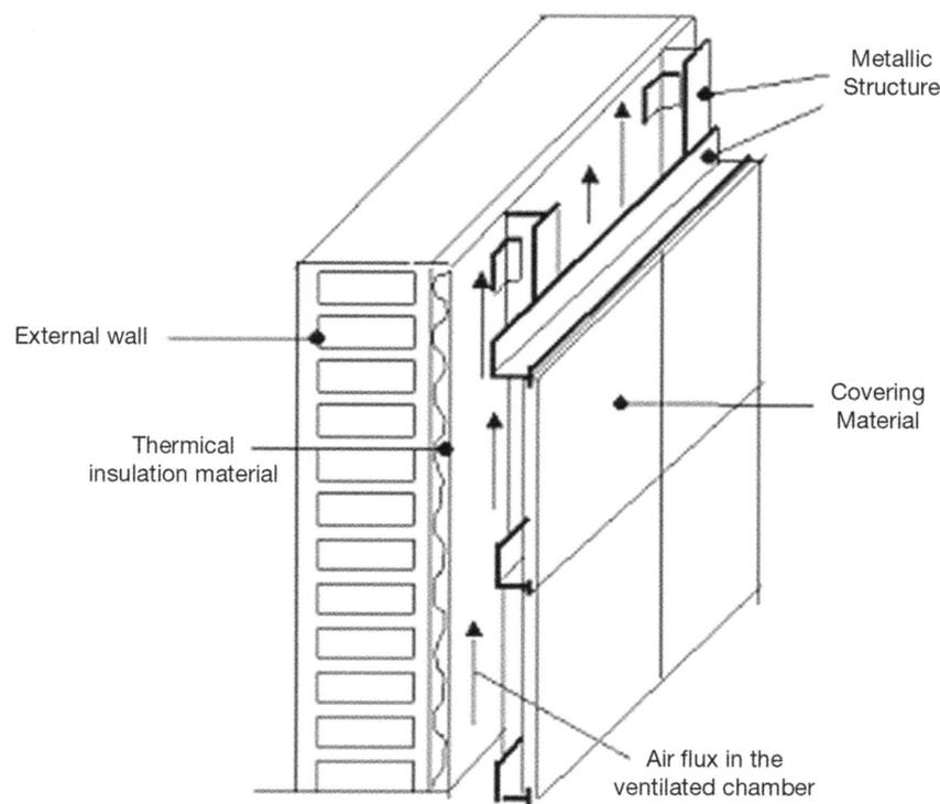
Figure 1. Scheme of ventilated facade covering system.
