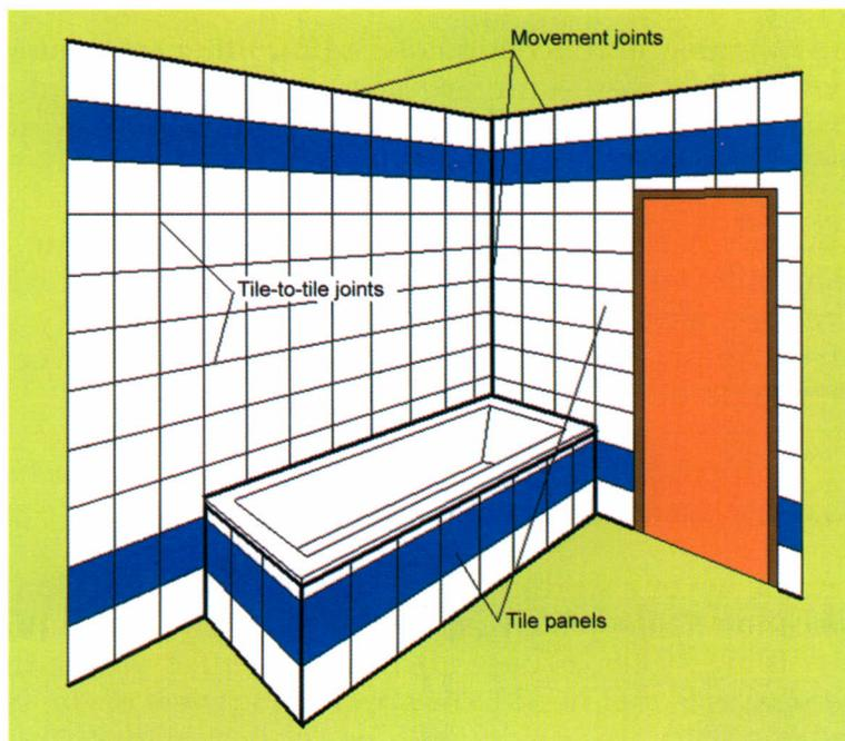
Figure 1. Schematic illustration of the "fair face" of a tiling system on a vertical facing
