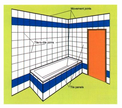
*Figure 1. Schematic illustration of the "fair face" of a tiling system on a vertical facing*
