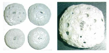
*Figure 1. The final products showing the expansion obtained with the addition of silicon carbide to a glaze waste at 1 wt% (bottom, left), 3 wt% bottom, right), 6 wt% (top, right) and 12 wt% (top, left). In the detail, the sample is shown with 12 wt% silicon carbide.*
