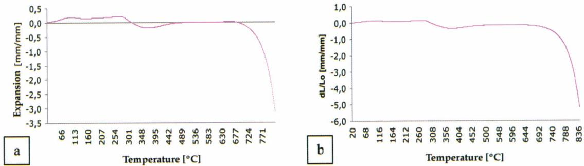
Figure 1. Expansion curves for (a) sample 1 (1 wt% zirconia) and (b) sample 5 (24 wt% zirconia).
