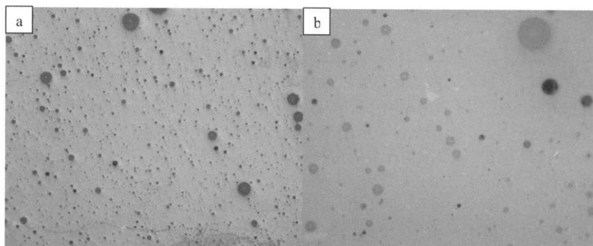
Figure 3. Sample micrographs (12 wt% de zirconia) (a) 50x magnification; (b) (100x) magnification.
