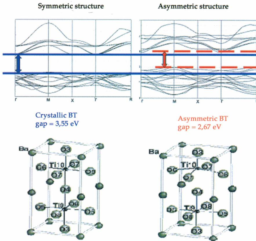
Figure 1. Band structures of BT. (a) crystalline. (b) asymmetric
