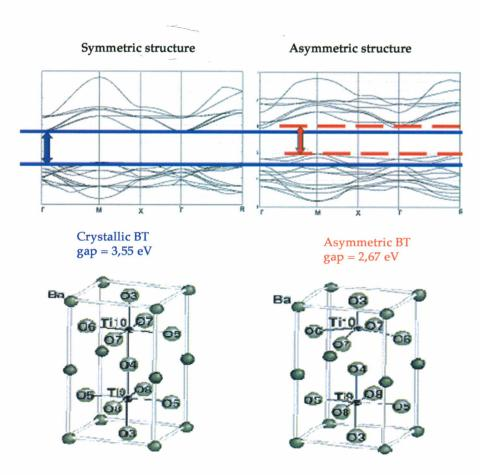
*Figure 1. Band structures of BT. (a) crystalline. (b) asymmetric*
