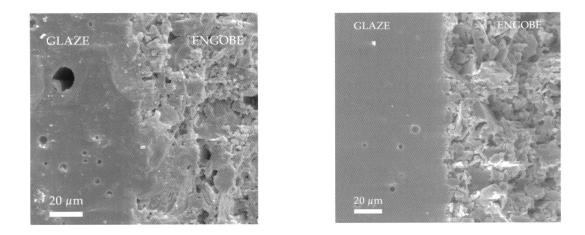
Figure 1. Interface of the sample that displayed no flaking (a) and that displayed flaking (b).
