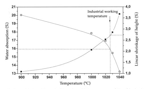
*Figure 2. Vitrification behaviour of the engobe of the product exhibiting a proneness to flaking of the glaze layer.*
